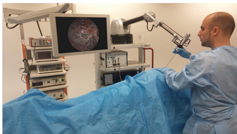
FIGURE 2.2: A comanipulated set-up for foetus surgery [57]
