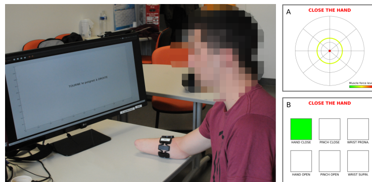
Figure 4.10: Left: amputated participant equipped with the MyoBand during the experiment. Right: View of the two different graphical interfaces used during the experiments. Top: Pattern Similarity Biofeedback GUI used with Group A (PSB-group) and amputated participant. Bottom: Raw-output feedback GUI used with Group B (RF-group).
