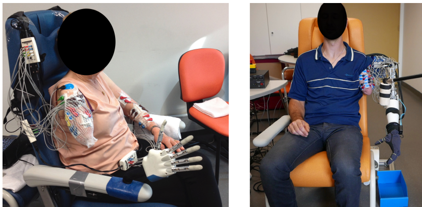
Figure 1.7: Experimental setups used to test, with transhumeral amputees, the control approach based on the decoding of the myoelectric patterns associated to the mobilization of the phantom limb, consequences of the neuromuscular reorganizations. Left: setup dedicated to the control of a polydigital hand. Right: setup dedicated to the control of an arm to perform functional tasks.
