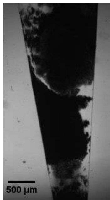
Figure 80 Formation of biofilm by Bacillus Cereus in the matrix of magnetic beads after one night of medium percolation at 37 °C
