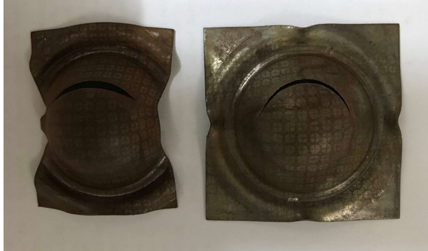
Figure 90. St-14 specimens after the test for mild steel St St-14
