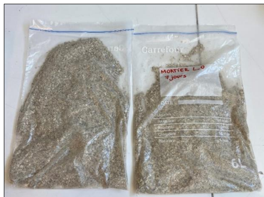
Figure 4-2 – Saturation of aggregate in hermetic bags 24 hours before mixing.
