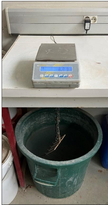
Figure 2-12 - Hydrostatic weighing device.
