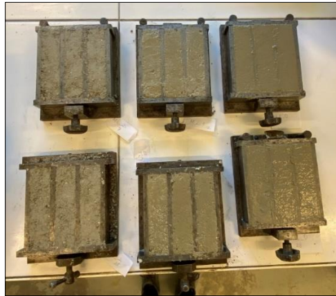
Figure 4-3 – 40 x 40 x 160 mm moulds filled with fresh mortar just after mixing.
