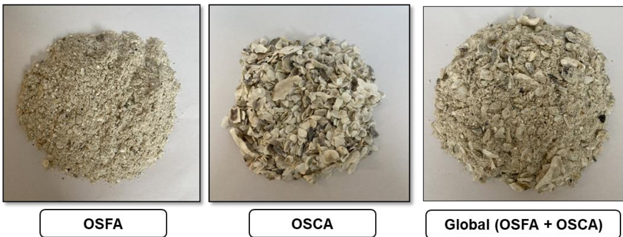
Figure 3-22 – OSFA (Oyster shell fine aggregate), OSCA (Oyster shell coarse aggregate) and Oyster shell global aggregate (mixture of OSFA + OSCA).
