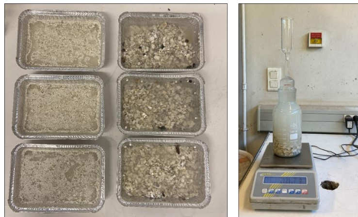
Figure 2-5 – Saturation of test specimens prior pycnometer method for oven-dried density test.
