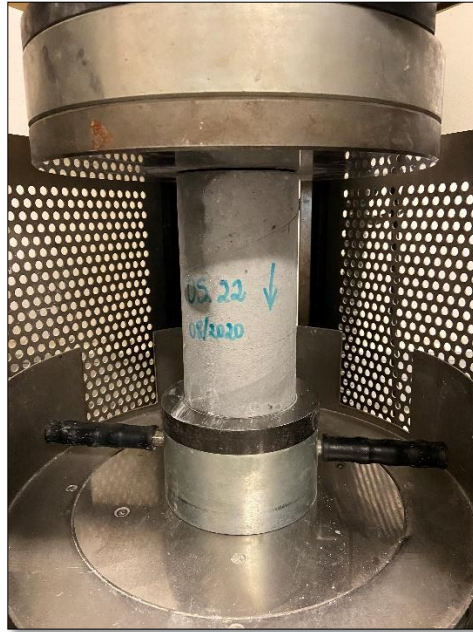
Figure 2-7 – Oyster shell concrete specimen placed in the machine for compressive test.
