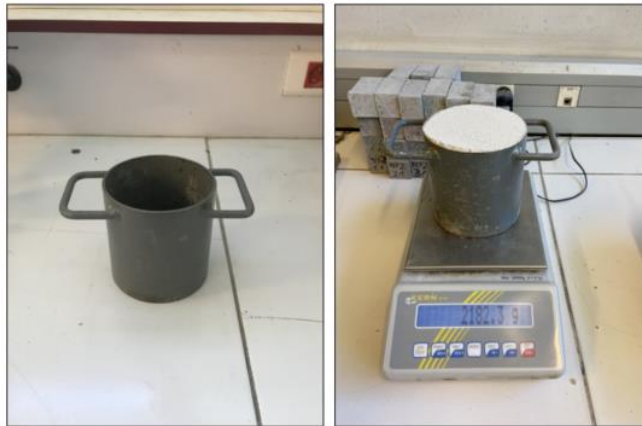
Figure 2-4 – Empty container (left), filled container with crushed oyster shells (right) used for the loose bulk density test.
