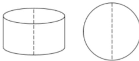
Figure 2-16 – Lengthwise sawn diagram on the cylinder 110x50 mm.
