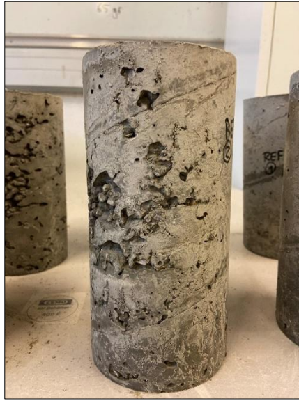
Figure 5-6 - Effect of the higher air entrapped in the CAC – NPA specimen.
