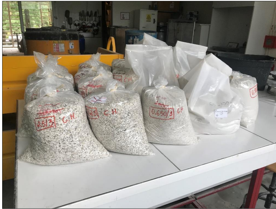
Figure 3-3 – Storage of crushed OS by particle groups in the laboratory.
