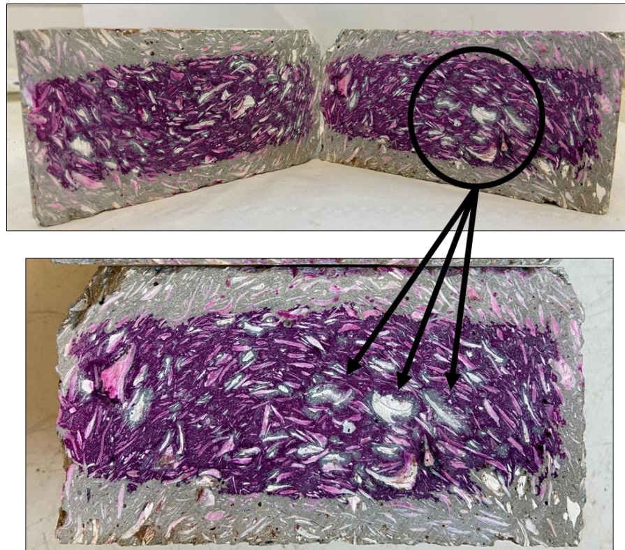
Figure 5-26 – pH \leq 9 \pm 1 zones around crushed oyster shell aggregates in the non-carbonated zone of OSC.
