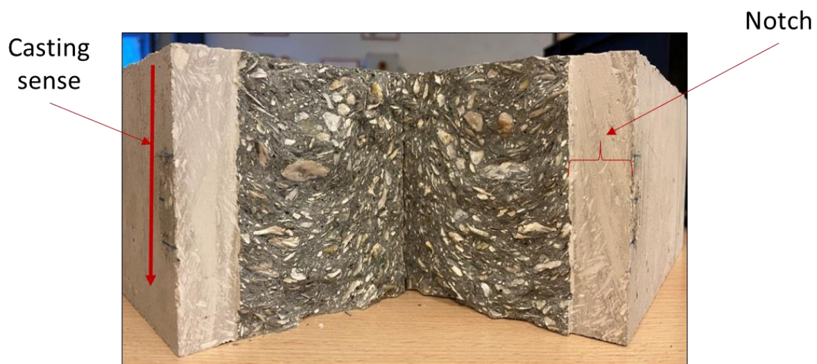
Figure 5-11 – OSC specimen after being tested for flexural strength.
