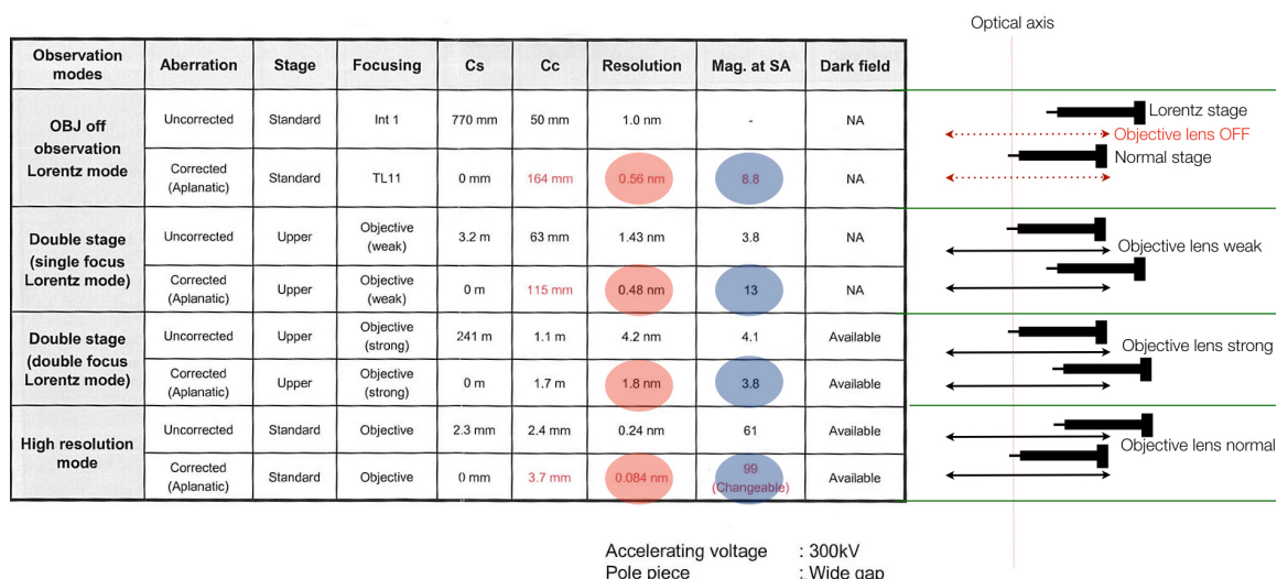
Figure 1.26 Summary of the optical properties offer by the four I2TEM imaging modes either non-corrected or using the aplanatic corrected B-COR properly aligned. From top to down : Lorentz TL_{11} mode with sample inserted inside normal stage, Lorentz single focus mode, Lorentz double focus mode and finally the normal (or high resolution) mode.
