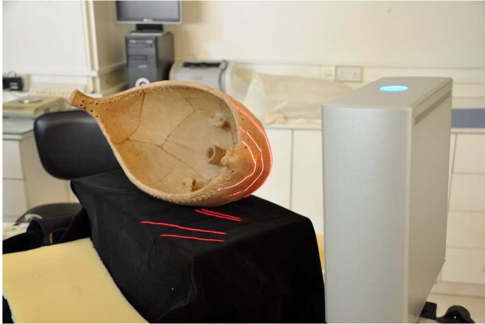
Figure 4.19: Acquisition of the Kazafani boat using NextEngine®LaserScanner.
