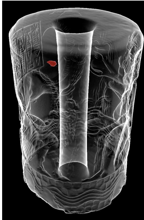
Figure 4.9: Model obtained from Computed Tomography. We can barely recognize the two kneeling figure because of the high noise produced by this technique.
