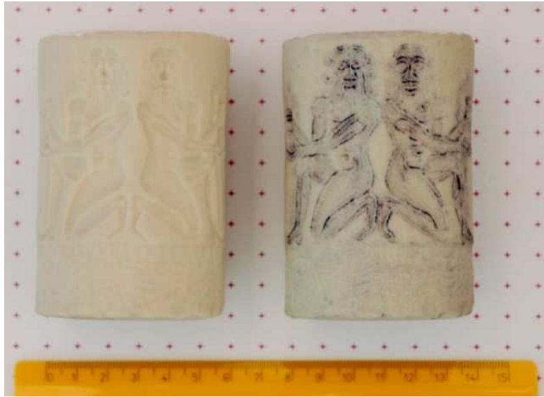
Figure 4.12: Two rapid prototyping reproductions, (left) done with the standard rapid prototyping technique; (right) with an automatic colour enhancement algorithm that put in evidence the small features of the seal using the technique proposed in [Cignoni et al., 2008a]; this recently proposed approach allows for the obtention of a better readability of the shape of the objects reconstructed using standard rapid prototyping techniques.
