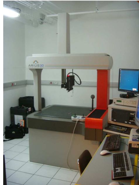
Figure 3.6: Arius3D setup at C2RMF. (left) schema representing the acquisition process. (right) the CMM and the laser head. The laser sources are hidden below the CMM for security reasons. On the right we can distinguish the dedicated unit for the CMM and laser real time acquisition, colour calibration and synchronization.
