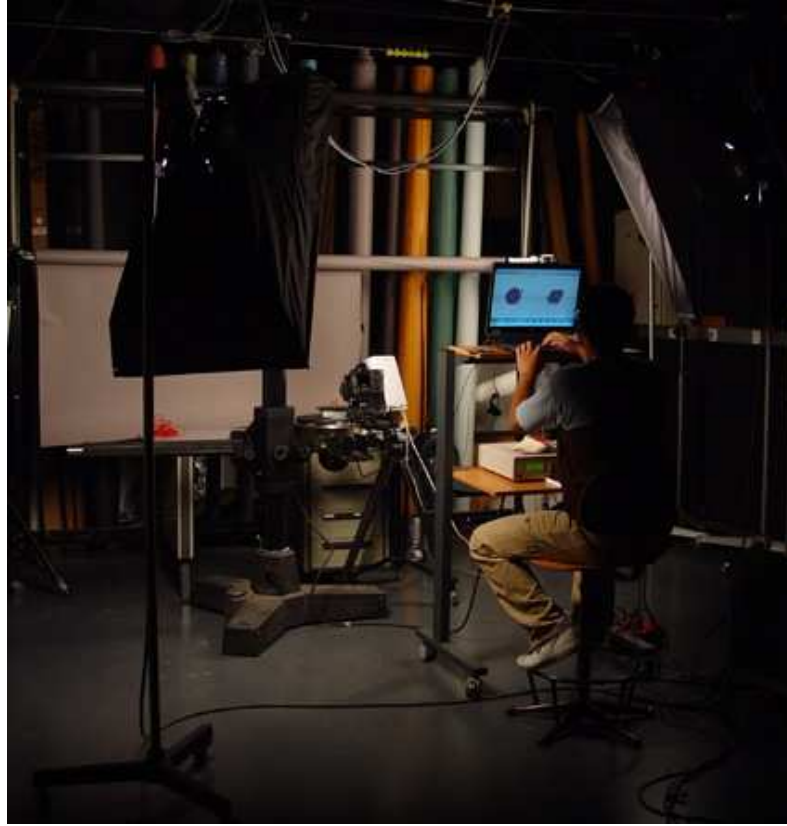
Figure 3.9: set up for “shape from silhouette” acquisition method at the C2RMF. In the centre of the photo the object and the camera are placed. The camera must not project any shadow in the acquisition area. The two light diffusers are covered with a polarized filter, to limit the backscattering from the object surface and the background is chosen to be of high contrast with the object itself. On the right side, the operator is handling the photographic and the 3D acquisition while using the turn table micro-controller.
