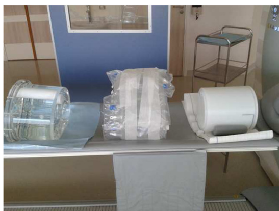
Figure 1. Phantoms used to derive the experimental relationship between NEC and SNR. Only the central part was centered in the FOV of the PET system. The two phantoms located on both sides of the central phantom simulated activity outside the FOV.
