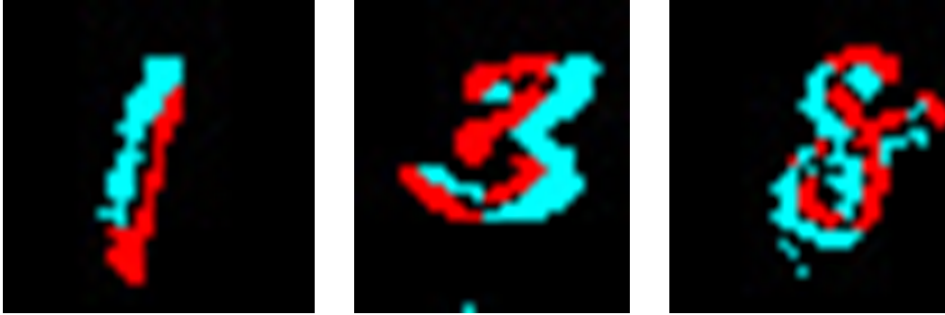
Figure 5.1: Samples of N-MNIST saccades snapshots in 2-D format. Black regions indicate no events, red indicates ON events, and blue indicates OFF events.
