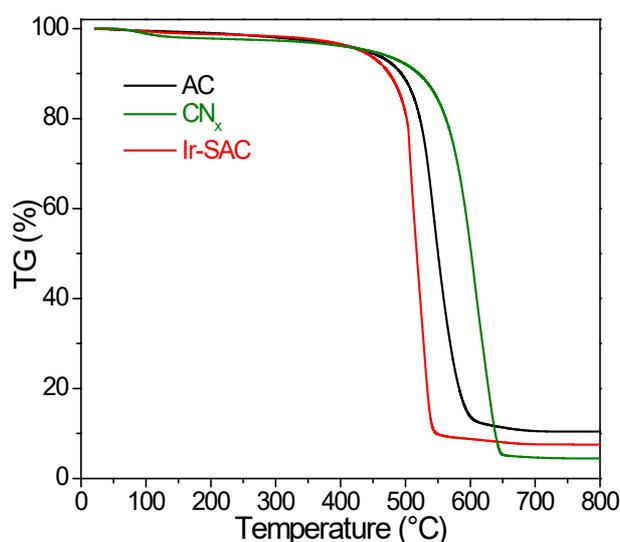
Figure 4. 9: TGA under dry air flow of pristine AC,  $CN_x$  and Ir-SAC.
