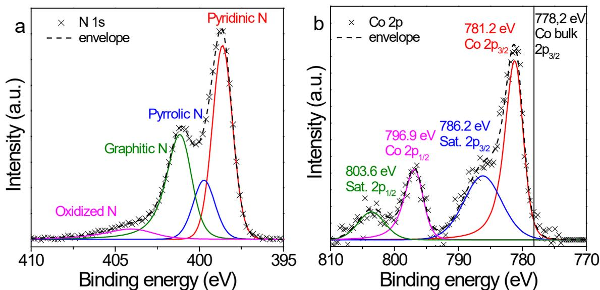
Figure 5. 4: a) N 1s and b) Co 2p XPS spectra of 1.0-Co-AC; The black line at 778.2 eV is the binding energy of Co bulk 2p<sub>3/2</sub> taken from literature.<sup>6</sup>
