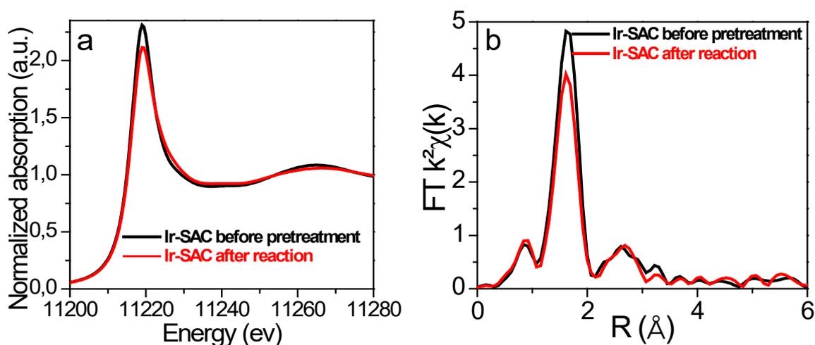
Figure 4. 19: a) XANES spectra at the Ir L<sub>3</sub>-edge of Ir-SAC before pretreatment and after reaction; b) Fourier transform of k<sup>2</sup>-weighted Ir L<sub>3</sub>-edge EXAFS data.
