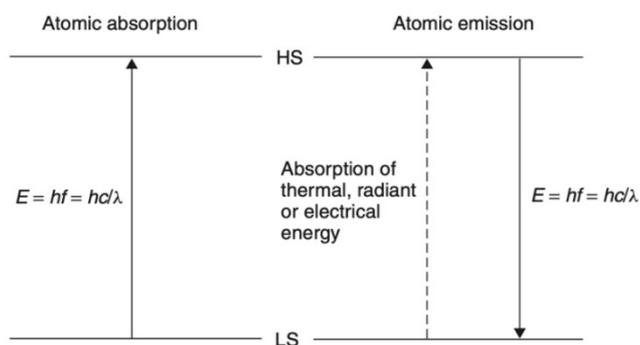
Figure 2. 13: Schematic representation of atomic absorption and atomic emission energy transitions: LS, lower-energy state or ground state; HS, higher-energy state.<sup>15</sup>
