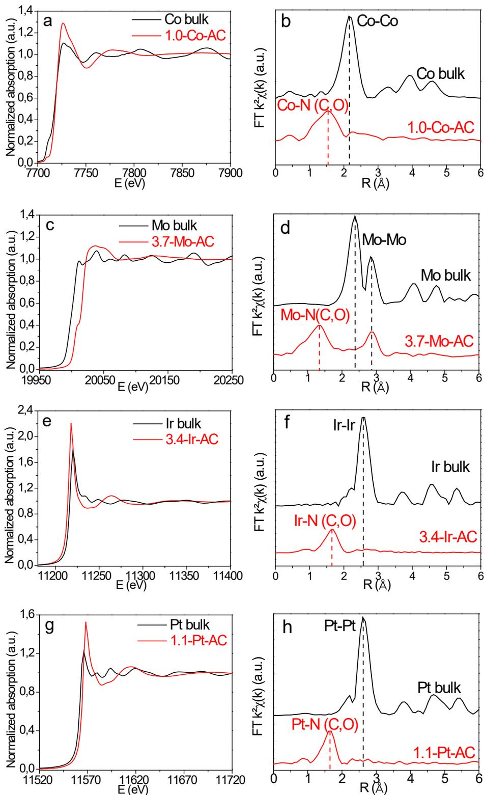
Figure 5.5: XANES spectra at the, a) K-edge of Co bulk (black) and 1.0-Co-AC (red), c) K-edge of Mo bulk (black) and 3.7-Mo-AC (red), e)  $L_3$ -edge of Ir bulk (black) and 3.4-Ir-AC (red), and g)  $L_3$ -edge of Pt bulk (black) and 1.1-Pt-AC (red); their corresponding Fourier Transform, b)
