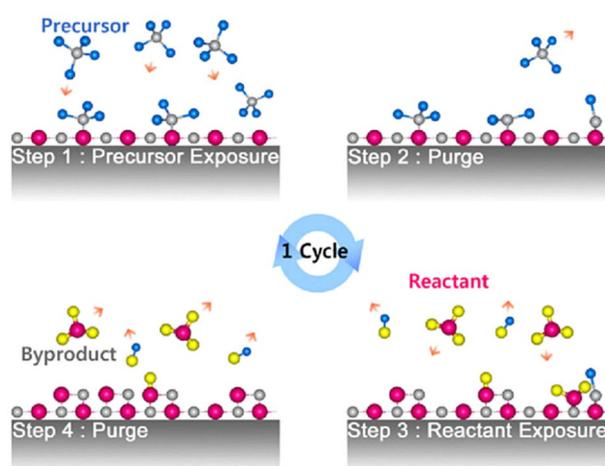
Figure 1. 15: Schematics showing the different steps of the ALD process for SAC preparation.<sup>77</sup>
