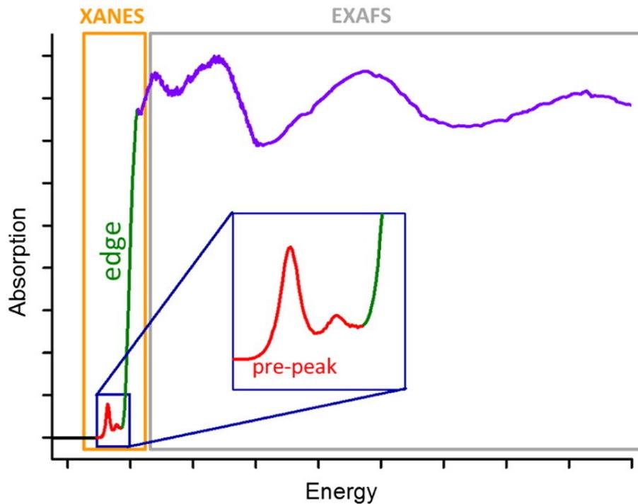
Figure 2. 12: X-ray absorption spectrum showing the X-ray absorption region near edge structure (XANES) including the pre-edge feature and extended X-ray absorption fine structure (EXAFS) region.<sup>7</sup>
