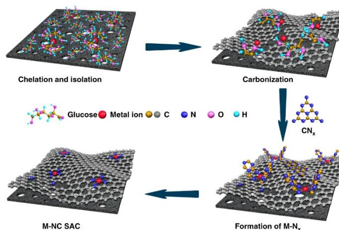
Figure 1. 16: Synthesis of M-NC SACs dispersed on carbon based support.<sup>79</sup>
