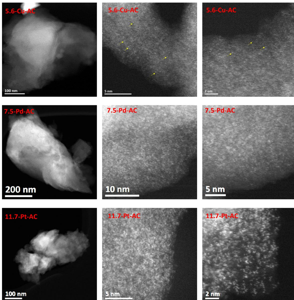
Figure 5. 8: HAADF-STEM images of 5.6-Cu-AC, 7.5-Pd-AC and 11.7-Pt-AC.
