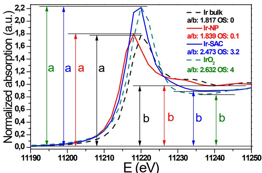
Figure 4. 15: XANES spectra of Ir bulk (black), Ir-NP (red), Ir-SAC (blue) and IrO<sub>2</sub> (green) showing the difference in peak heights for these samples, and the parameters *a* and *b* used for the assessment of the oxidation state.
