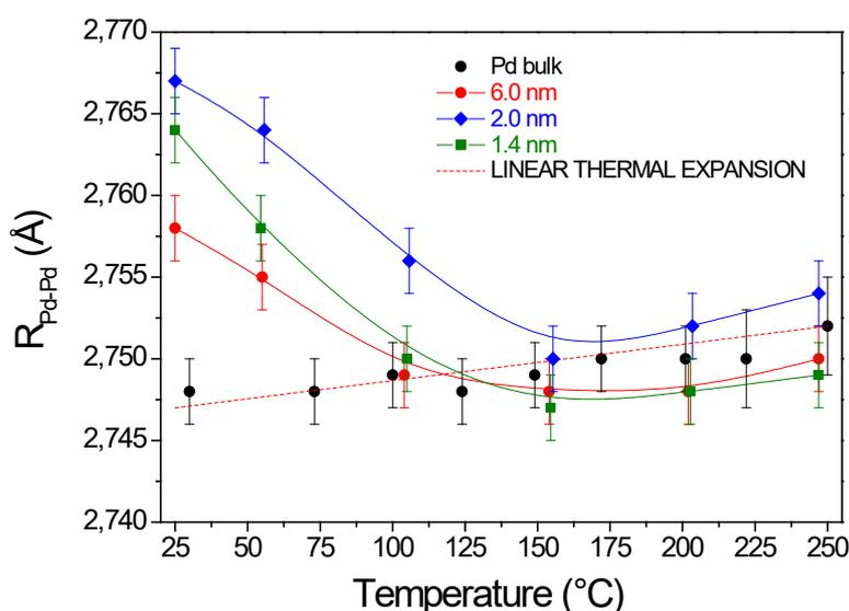
Figure 3. 13: The thermal variation of  $R_{\text{Pd-Pd}}$  in *in situ* XAS under He flow during heating to 250 °C for desorbed Pd bulk, 6.0 nm, 2.0 nm and 1.4 nm Pd ( $10 \text{ }^\circ\text{C/min}$ ).
