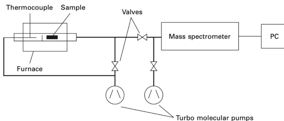
Figure 2. 16: Schematic illustration of thermal desorption spectroscopy apparatus.<sup>18</sup>
