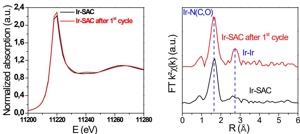
Figure 4. 25: a) XANES spectra at the Ir L<sub>3</sub>-edge of Ir-SAC (black) and Ir-SAC after 1<sup>st</sup> cycle (red) and b) their corresponding Fourier transform. For the sake of comparison, FT have been stacked.
