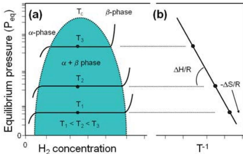
Figure 1. 5: a) Pressure–concentration–isotherms plots and b) a van't Hoff curve (logarithm of the equilibrium or plateau pressure against the reciprocal temperature).<sup>24</sup>
