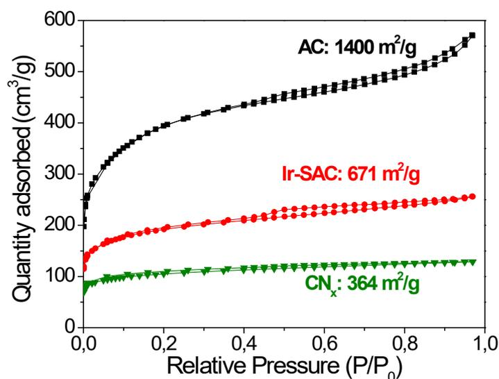
Figure 4. 3: Liquid N<sub>2</sub> adsorption/desorption curves of AC, CN<sub>x</sub>, and Ir-SAC, determined at ICMPE.
