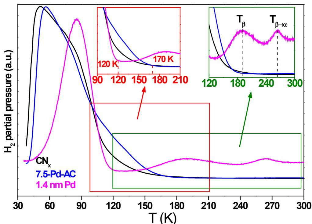
Figure 3. 28: Thermo-desorption spectra of  $CN_x$ , 7.5-Pd-AC and 1.4 nm Pd with a heating rate of 5 K/min.
