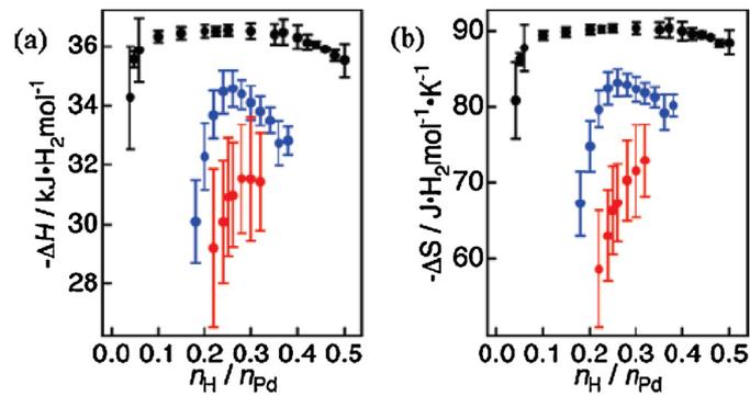
Figure 1. 9: Hydrogen concentration dependence of a) the heat of formation ( $-\Delta H$ ) and b) the standard entropy ( $-\Delta S$ ) for the phase transition  $\alpha \rightarrow \beta$ : bulk Pd (black), 7 nm (blue) and 2.6 nm (red) Pd nanoparticles confined into PVP polymer.<sup>37</sup>
