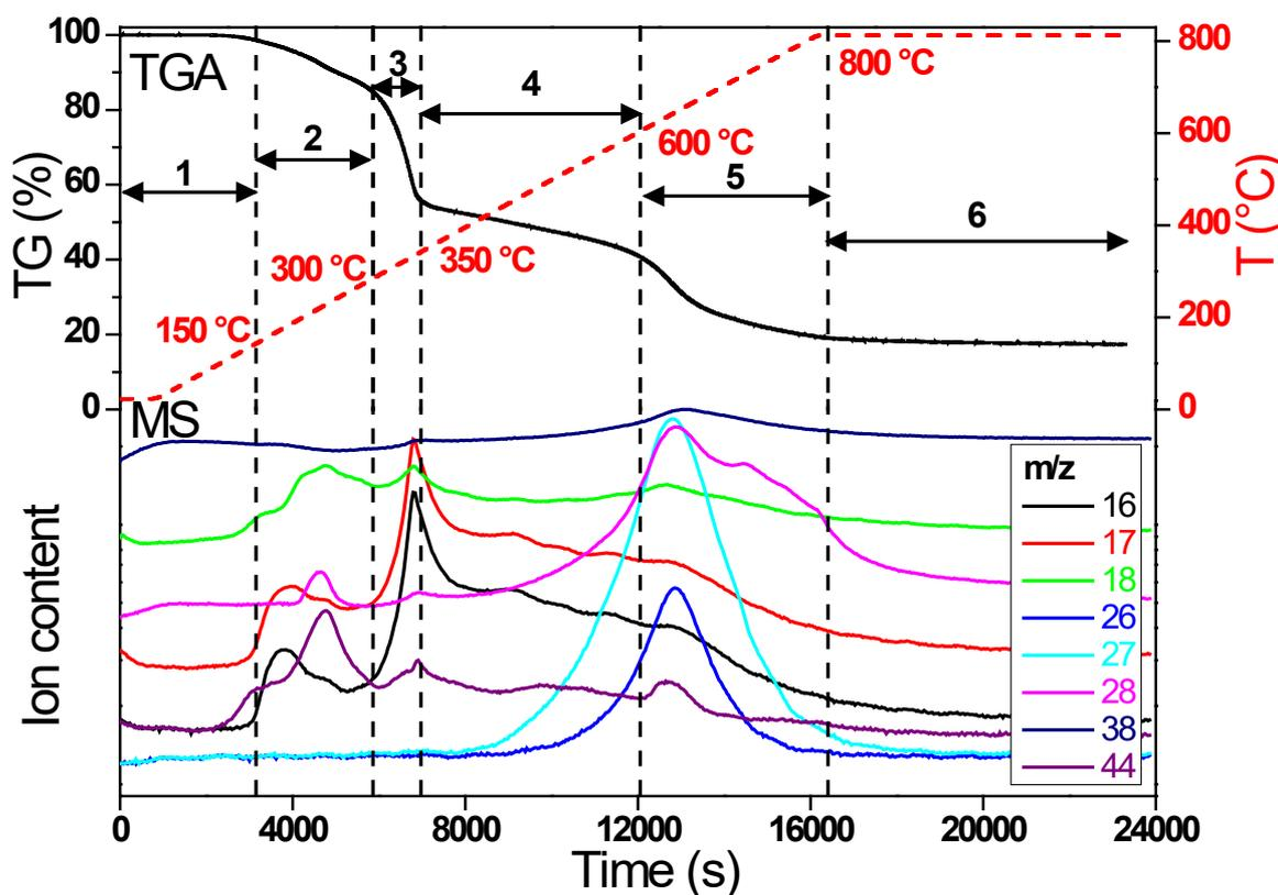
Figure 4. 7: TGA-MS data of the mixture of IrCl<sub>3</sub>, AC, EDTA and melamine (0.3 wt.% IrCl<sub>3</sub>, 12.5 wt.% AC, 25 wt.% EDTA and 62.5 wt.% melamine), the final product after TGA is Ir-SAC.
