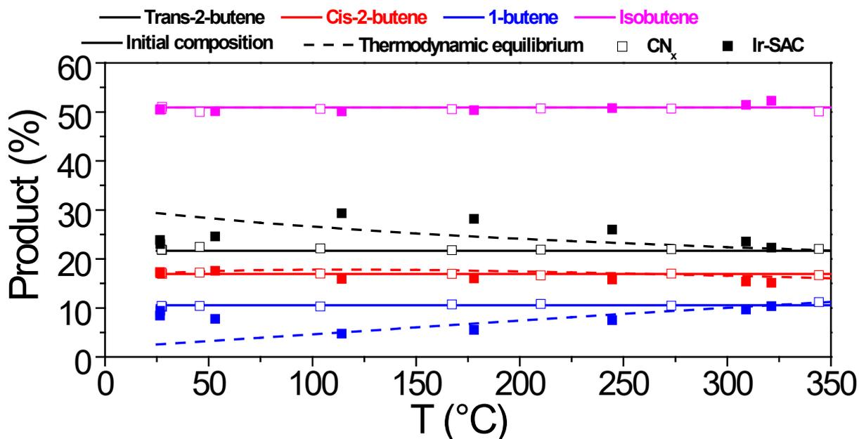
Figure 4. 12: Isomerization of butenes over Ir-SAC and  $CN_x$ . The solid line represents the initial composition of butenes, the dashed line represents the thermodynamic equilibrium composition as a function of temperature (without considering the isobutene), the void square represents the results of  $CN_x$  and the solid square represents the results of Ir-SAC.
