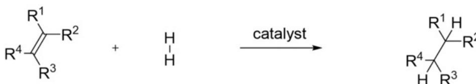
Figure 1. 3: Schematic representation of hydrogenation.<sup>13</sup>
