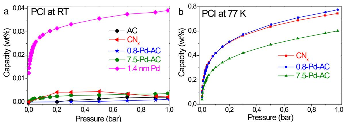
Figure 3. 26: Pressure-composition-isotherms curves of a) AC, 1.4 nm Pd, 0.8-Pd-AC and 7.5-Pd-AC at room temperature and b) CN<sub>x</sub>, 0.8-Pd-AC and 7.5-Pd-AC at cryogenic temperature (77K).
