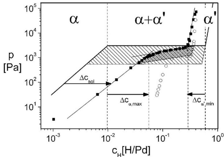
Figure 1. 8: Pressure-composition-isotherms for Pd bulk (straight lines) and clusters (full squares indicate absorption and empty circles correspond to desorption). The  $\alpha$  phase corresponds to a solid solution and the  $\alpha'$  (or  $\beta$ ) is the hydride phase.<sup>36</sup>
