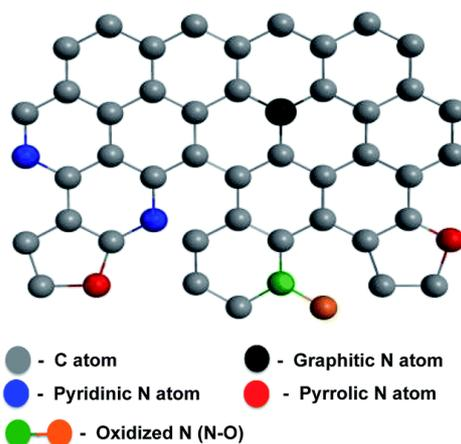
Figure 1. 13: Schematic representation of different types of N atoms (graphitic, pyridinic, pyrrolic and oxidized N) in nitrogen-doped carbon.<sup>68</sup>
