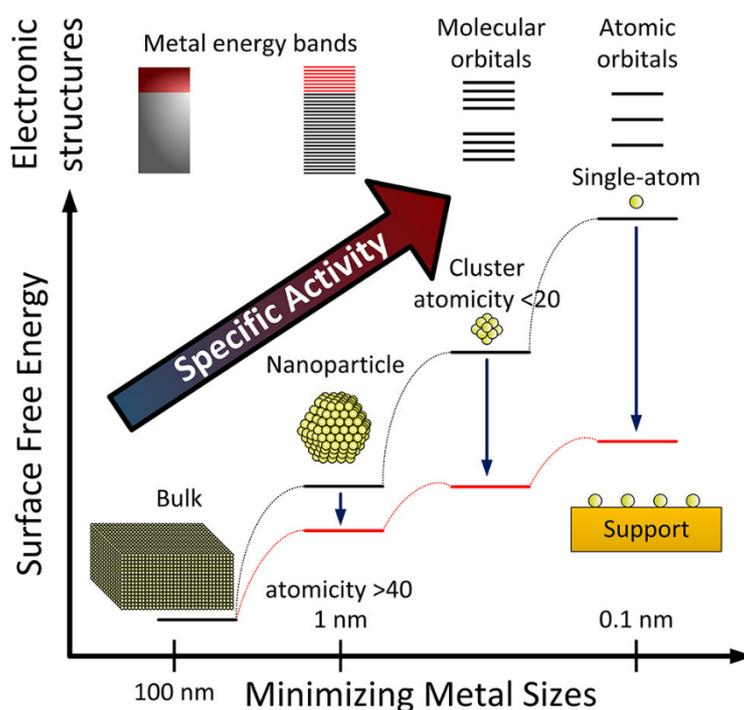
Figure 1. 6: Illustration of the downsizing metal sizes and evolution of the geometric configuration, electronic structure and surface free energy as the size of metal particles decreases.<sup>28</sup>
