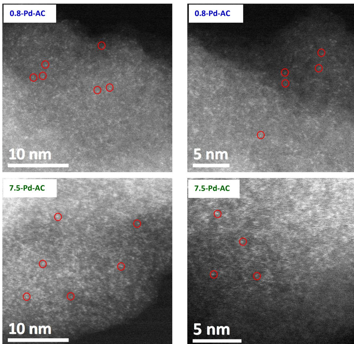
Figure 3. 23: HAADF-STEM images of 0.8-Pd-AC and 7.5-Pd-AC, the bright spots in the red circles are Pd atoms.
