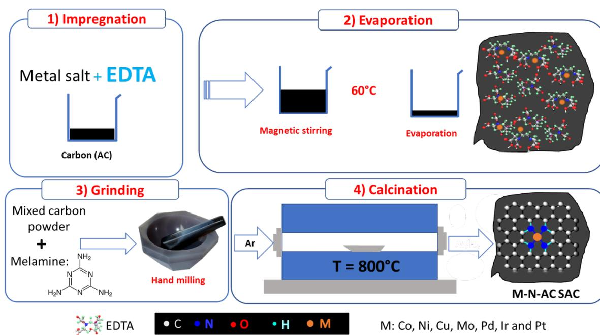
Figure 2. 2: Schematic illustration of the synthesis of metal SACs supported on porous carbon materials.
