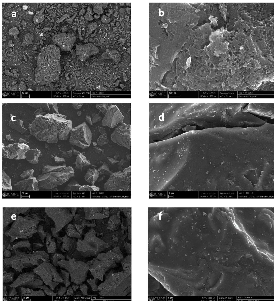
Figure 3.25: SEM images of a, b) AC; c, d) CN<sub>x</sub> and e, f) 0.8-Pd-AC.
