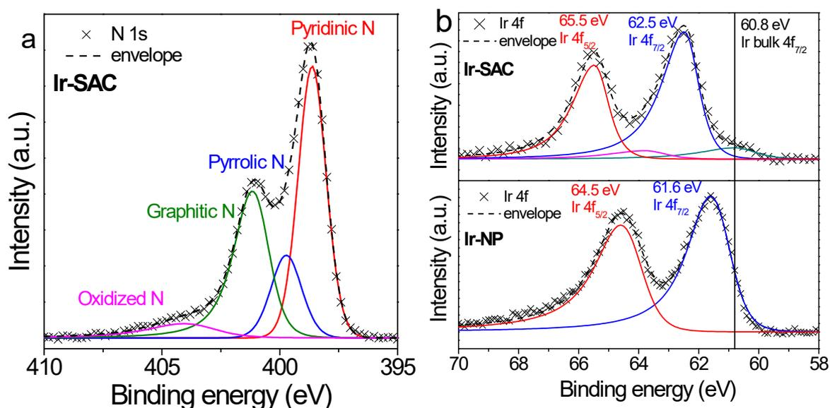
Figure 4. 6: a) N 1s XPS spectrum of Ir-SAC and b) Ir 4f XPS spectra of Ir-SAC and Ir-NP; The black line at 60.8 eV is the binding energy of Ir bulk 4f<sub>7/2</sub> taken from literature.<sup>5</sup>
