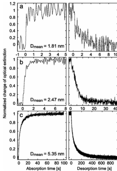
Figure 1. 10: Experimental hydrogen absorption (left column) and desorption (right column) kinetics for three mean diameters: a) 1.81 , b) 2.47, and c) 5.35 nm of Pd nanoparticles.<sup>40</sup>
