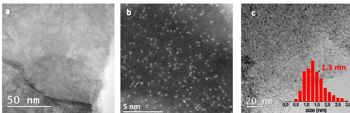
Figure 4. 2: a) TEM image of 1.0-Ir-AC, b) HAADF-STEM image of 1.0-Ir-AC, and c) TEM image of 3.7-Ir@AC-700.
