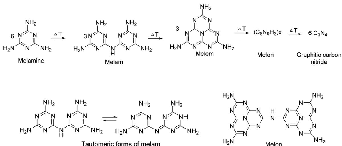
Figure 4. 8: Thermal decomposition of melamine and the formation of graphitic carbon nitride.<sup>7</sup>
