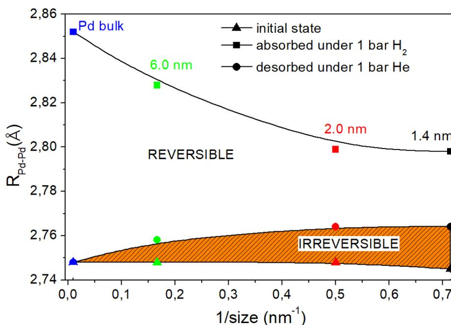
Figure 3. 11: The variation of  $R_{Pd-Pd}$  as function of the inverse of particle size for several sizes of Pd bulk, 6.0 nm, 2.0 nm and 1.4 nm Pd as initial state (triangle), absorbed state under 1 bar H<sub>2</sub> (square) and desorbed phase (circle).
