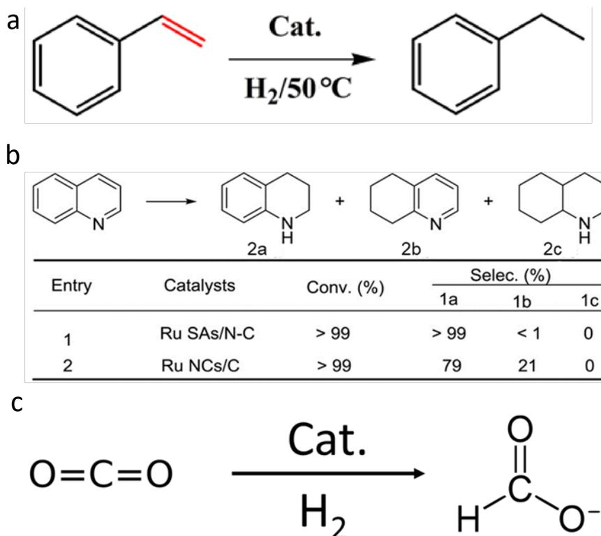
Figure 1. 22: a) Hydrogenation of styrene,<sup>78</sup> b) Hydrogenation of quinoline and Catalytic performance of Ru SACs and Nanoparticles catalysts,<sup>94</sup> and c) Hydrogenation of CO<sub>2</sub> to formate.
