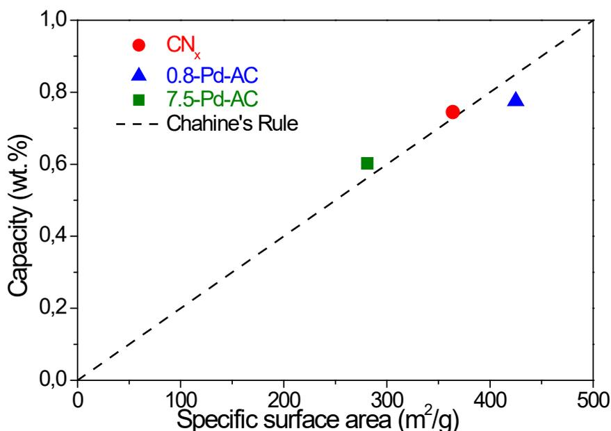
Figure 3. 27: Correlation between the BET surface area and the hydrogen storage capacity (at 1 bar H<sub>2</sub> and 77 K) of CN<sub>x</sub>, 0.8-Pd-AC and 7.5-Pd-AC. The dashed line represents Chahine's rule.
