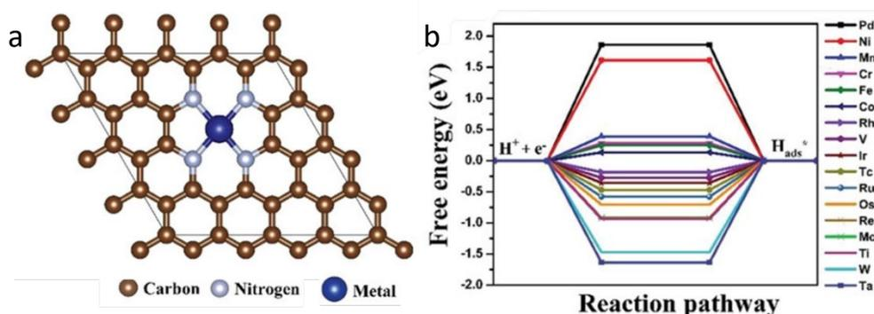
Figure 1. 21: a) Metal coordinated with four nitrogen atoms in graphene sheet. d) Gibbs free energy ( $\Delta G_H$ ) diagram for hydrogen adsorption reaction (Volmer reaction) toward a series of transition metals used as single atom catalysts.<sup>91</sup>
