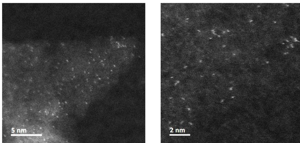
Figure 4. 10: HAADF-STEM images of Ir-SAC after H<sub>2</sub> treatment at 400 °C.
