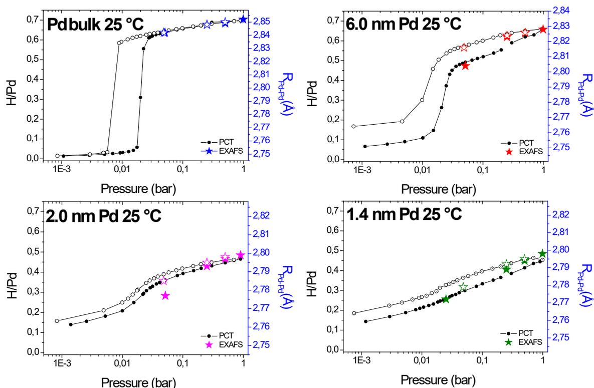
Figure 3. 10: Comparison between the PCI curves (expressed as H/Pd vs. Pressure) and the nearest Pd-Pd distances determined by EXAFS as function of H<sub>2</sub> pressure for Pd bulk, 6.0 nm, 2.0 nm and 1.4 nm Pd at 25 °C. Full and empty symbols stands for absorption and desorption, respectively.
