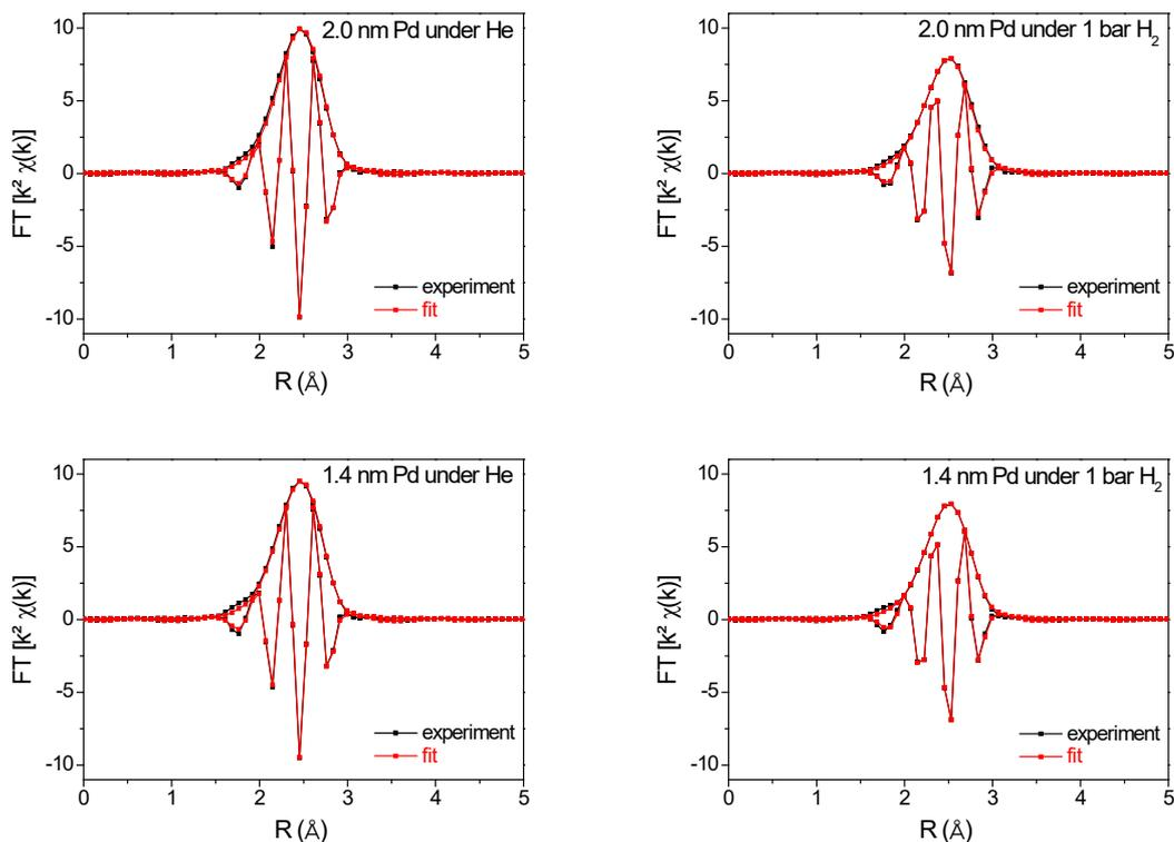
Figure 3. 9: Selected EXAFS refinements between FT (black) and fitted (red) for Pd bulk and 6.0 nm, 2.0 nm and 1.4 nm Pd under He and 1 bar  $H_2$  at room temperature.
