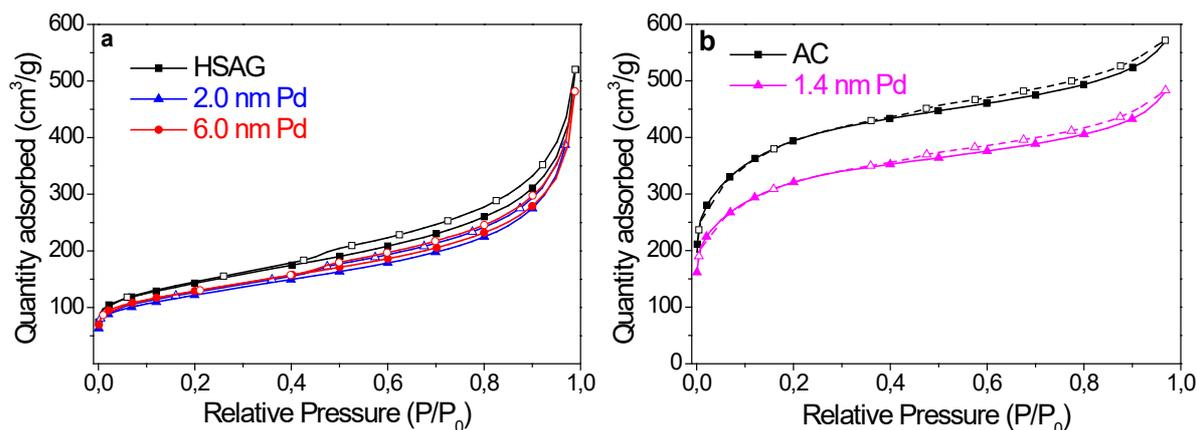
Figure 3. 4: N<sub>2</sub> adsorption/desorption curves at 77 K of (a) HSAG, 6.0 nm and 2.0 nm Pd, and (b) AC and 1.4 nm Pd.
