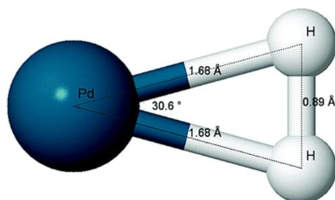
Figure 1. 20: Structure of the Pd(H<sub>2</sub>) complex as calculated by DFT, indicating bond lengths and angles.<sup>90</sup>
