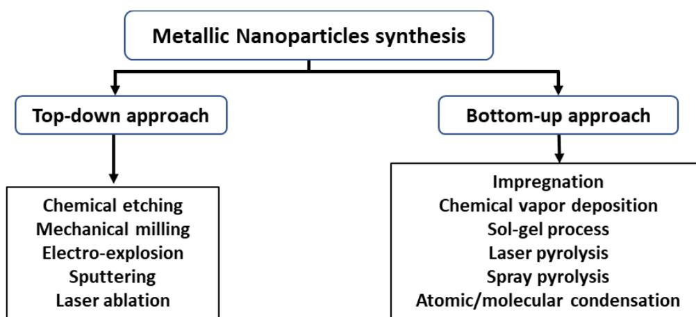
Figure 1. 7: Different synthesis approaches available for the preparation of metal nanoparticles.<sup>31</sup>
