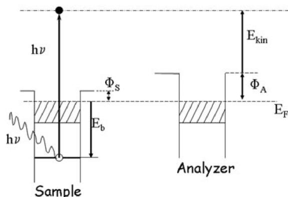
Figure 2. 10: Schematic explanation of relevant energy terms in XPS of solid surfaces.<sup>6</sup>
