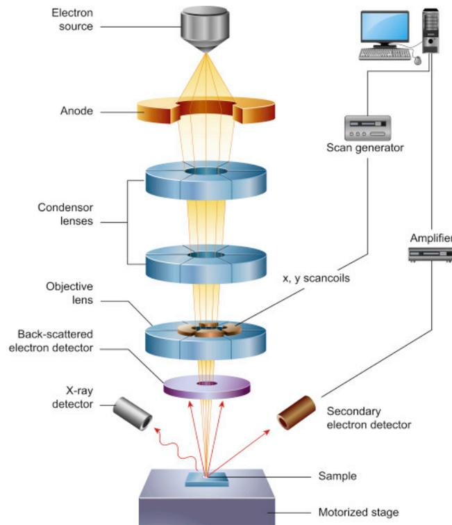
Figure 2. 4: Schematic diagram of an SEM microscope.<sup>2</sup>
