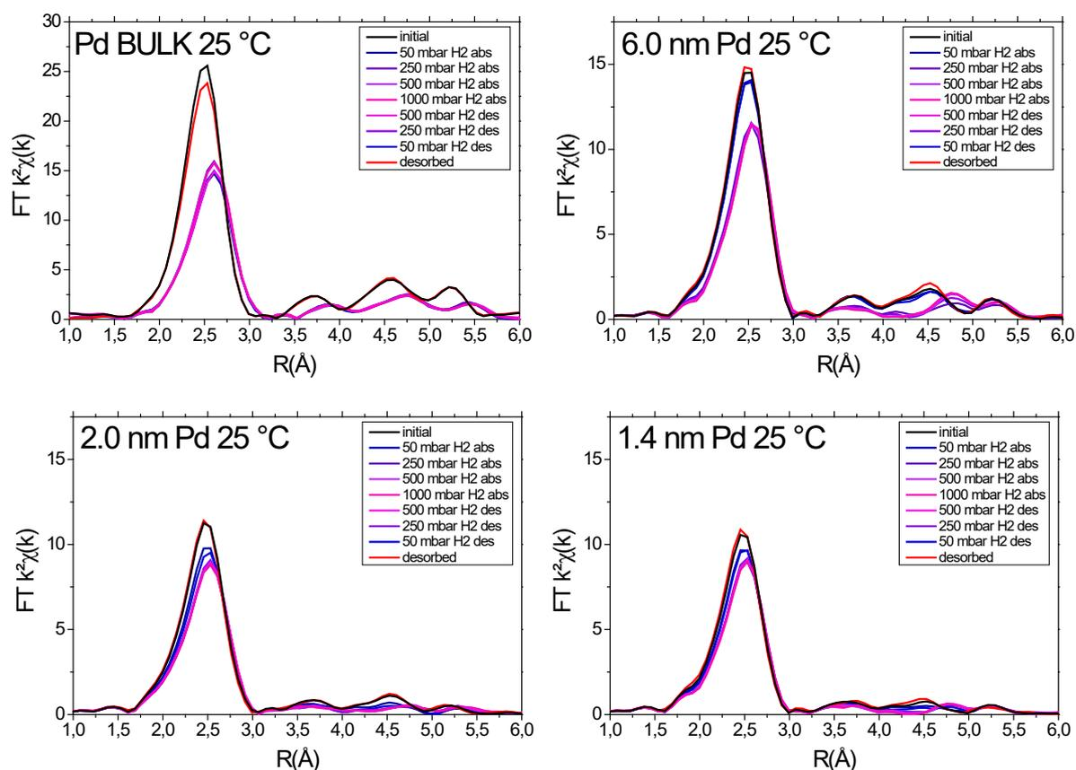
Figure 3. 8: FT of the EXAFS spectra ( $k^2\chi(k)$ ) for Pd bulk and 6.0 nm, 2.0 nm and 1.4 nm Pd under various partial pressures of H<sub>2</sub> at 25 °C.
