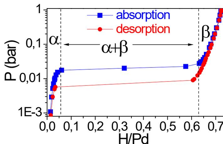
Figure 2. 15: Example of Pressure-Composition Isotherm of Pd bulk at RT.
