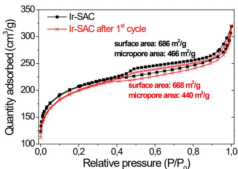
Figure 4. 23: Liquid N<sub>2</sub> adsorption/desorption curves of Ir-SAC and Ir-SAC after 1<sup>st</sup> cycle.
