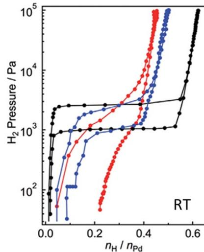
Figure 1. 11: Pressure-Composition-Isotherms curves at room temperature for Pd bulk (black) and Pd nanoparticles of size  $7.0 \pm 0.4$  nm (blue) and  $2.6 \pm 0.4$  nm (red).<sup>42</sup>
