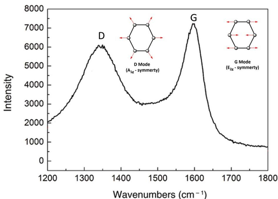
Figure 2. 9: Raman spectrum of activated carbon materials, collected with an excitation  $\lambda = 514\text{ nm}$ , and assignment of the main bands. The insets show a scheme of the vibrational modes associated with the two main bands.<sup>5</sup>
