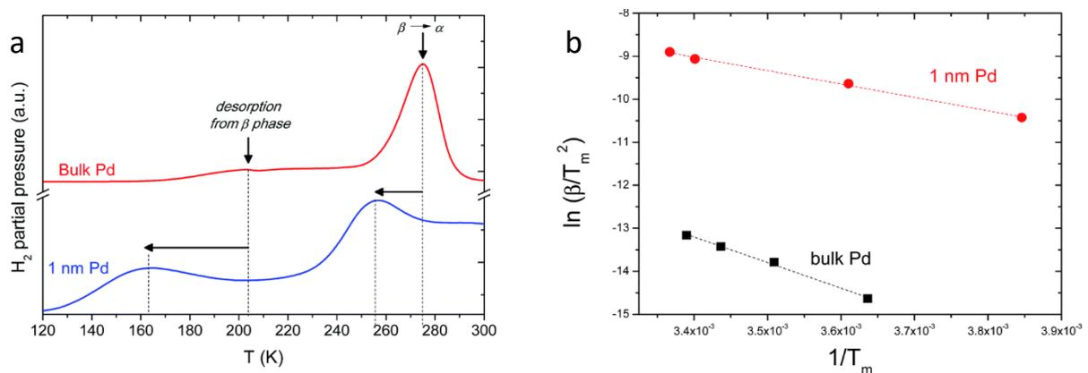
Figure 1. 12: a) Thermo-desorption spectra of the bulk and 1 nm Pd with a heating rate of 2 K/min and b) The Kissinger plots for bulk and 1 nm Pd.<sup>33</sup>
