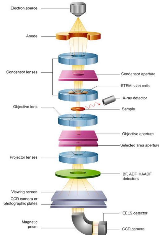
Figure 2. 5: Schematic of core components of a TEM microscope.<sup>2</sup>
