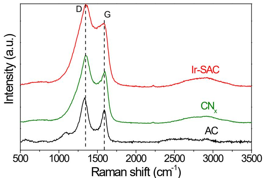
Figure 4. 5: Raman spectra of AC,  $CN_x$ , and Ir-SAC.
