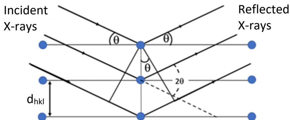
Figure 2. 3: Bragg reflection for X-ray diffraction.
