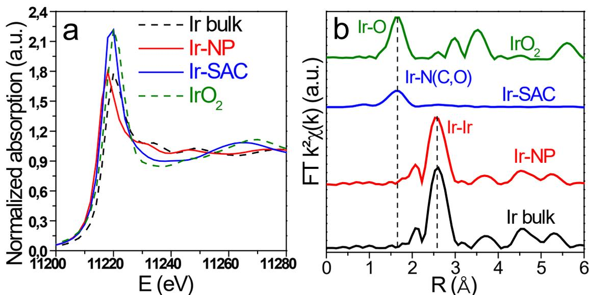
Figure 4. 14: a) XANES spectra at the Ir L<sub>3</sub>-edge of Ir bulk (black), Ir-NPs (red), Ir-SAC (blue) and IrO<sub>2</sub> (green) before reaction at RT, and b) their corresponding Fourier transform. For the sake of comparison, FT have been stacked.
