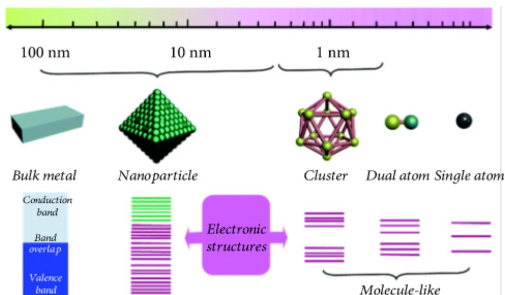
Figure 1. 1: Illustration of the downsizing metal sizes, and evolution of the electronic structures.<sup>3</sup>
