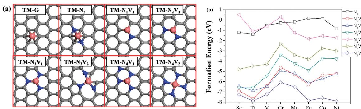
Figure 1. 14: a) Optimized structures and b) formation energies for N-doped graphene.<sup>69</sup>
