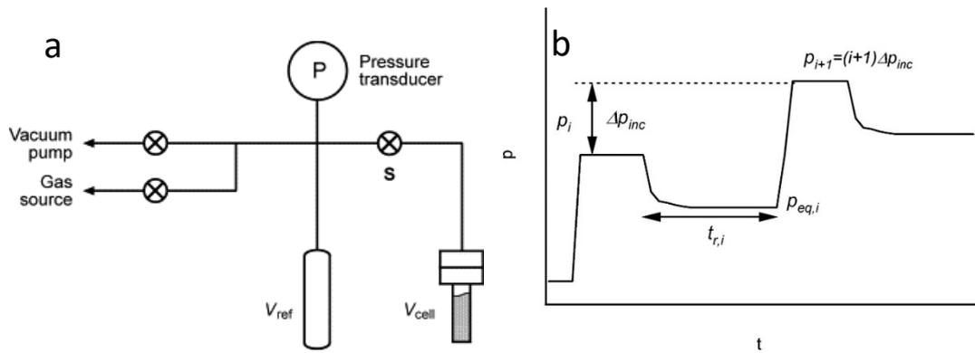
Figure 2. 14: a) Schematic representation of a Sievert's apparatus,<sup>16</sup> and b) Schematics of the measurement procedure in a Sieverts apparatus. The schematics illustrates the acquisition of point  $i+1$ .<sup>17</sup>
