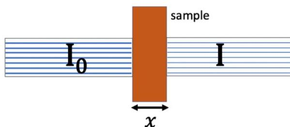
*Figure 2. 11: Incident and transmitted X-ray beams in the presence of a sample with  $x$  thickness.*
