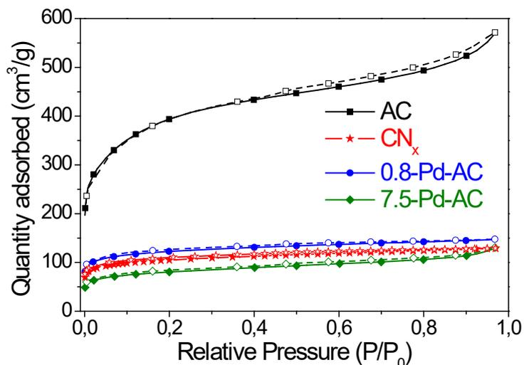
Figure 3. 24: Liquid N<sub>2</sub> adsorption/desorption curves of AC, CN<sub>x</sub>, 0.8-Pd-AC and 7.5-Pd-AC.
