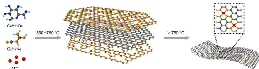
Figure 1. 17: Synthesis of M-NC SACs via one pot synthesis.<sup>81</sup>
