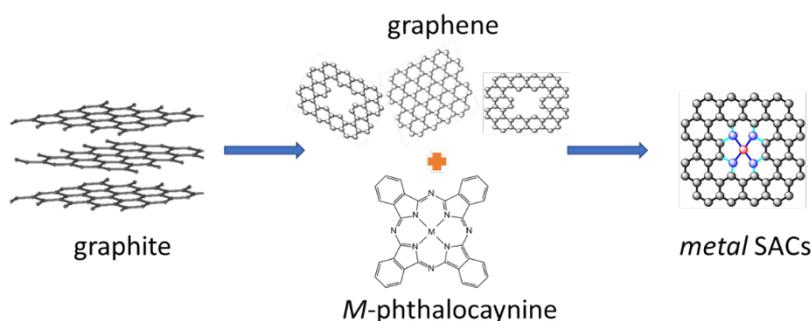
Figure 1. 19: Scheme of a proposed mechanism for synthesis of metal SACs via ball milling method.<sup>88</sup>
