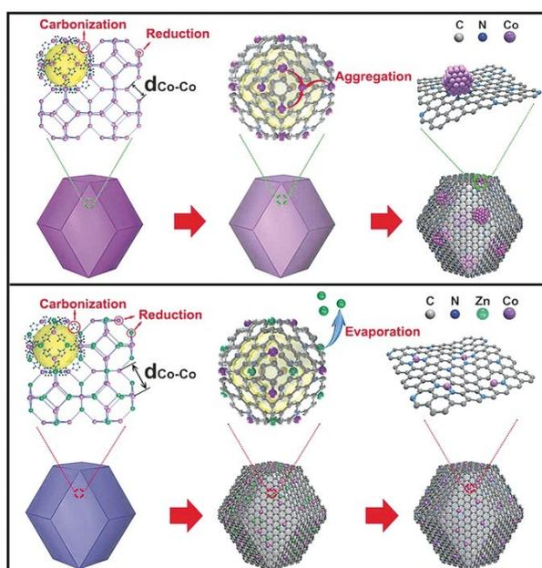
Figure 1. 18: The formation of Co Nanoparticles/N-C (top) and Co Single-atoms/N-C (bottom).<sup>85</sup>
