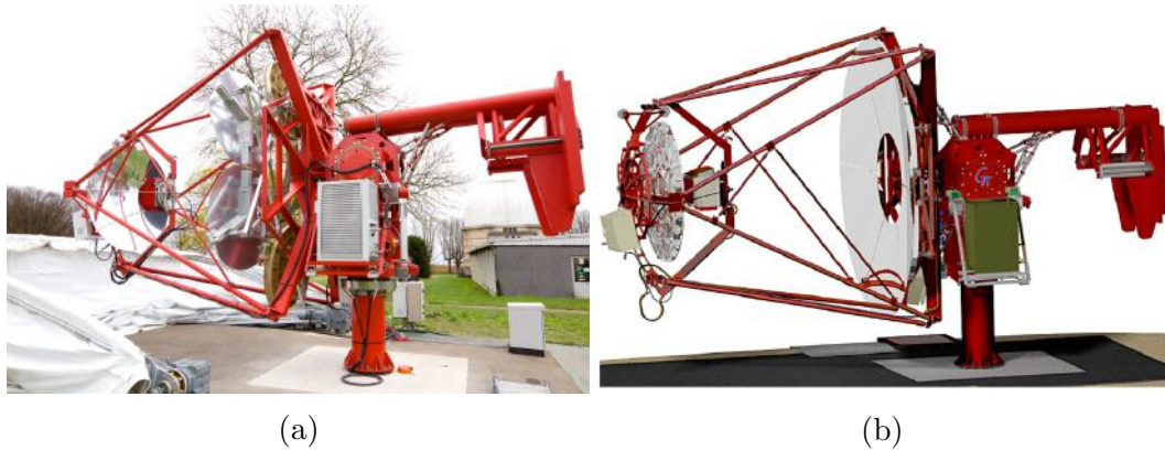
Figure 4.8: The GCT telescope. (a) is a picture of the GCT prototype built at the Observatoire de Paris in Meudon. (b) represents the final design of GCT proposed for CTA.
