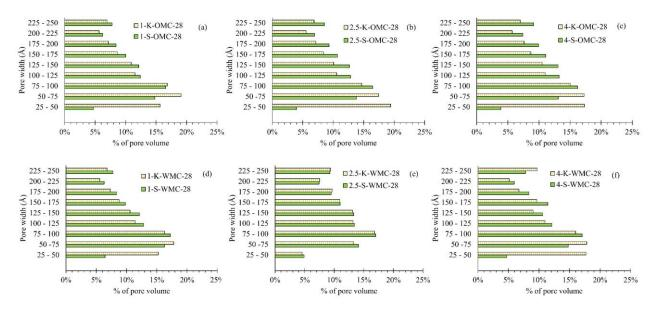
Fig. 4-6 Percentage of cumulative mesopores volume measured in 1%, 2.5%, and 4% lime-treated OMC, and WMC kneading and statically compacted specimens after 28 days (a-f) and 90 days (g-i) of curing at 20°C.
