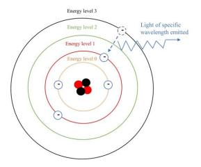
Fig. 2-7 Schematic diagram showing excitement of electrons, thus jumping to a high-level energy after absorbing energy, and again returning to the low-level energy by releasing light of specific wavelength (after Fassel and Kniseley, 1974).
