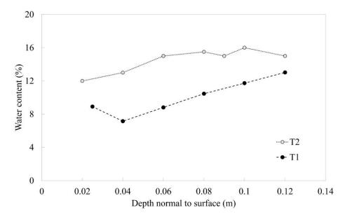
Fig. 3-7 Water content (%) measured on specimens sampled from the upper layer of the lime-treated embankment during deconstruction.
