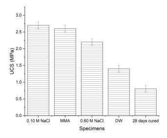
Fig. 7-2 Unconfined Compressive Strength obtained after 5 W-D cycles.
