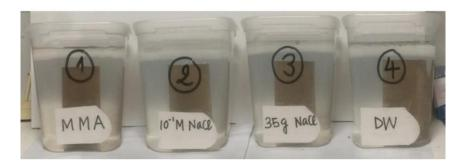
Fig. 7-1 Lime-treated specimens placed in four different fluids for 1st wetting during the W-D cycles.
