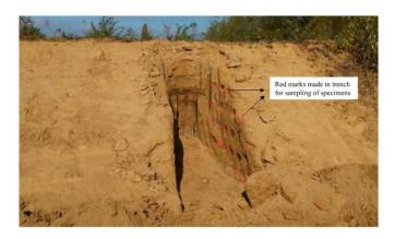
Fig. 3-1 Trench excavated in the lime-treated embankment (T2) for the sampling of specimens.
