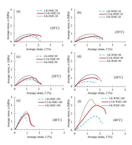
Fig. 4-1 Strength evolution of 1%, 2.5% and 4% lime-treated kneading compacted specimens at OMC-28 days (a), WMC-28 days (b), OMC-90 days (c), WMC-90 days (d), OMC-180 days (e), and WMC-180 days (f).
