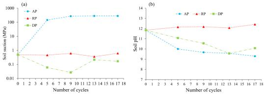
Fig. 6-3 Soil suction (a) and pH (b) measured in the initial and UCS subjected specimens during W-D/D-W cycles as per AP, RP, and DP testing conditions.
