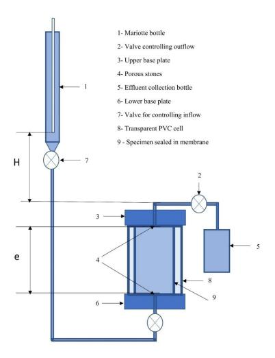
Fig. 2-5 Schematic diagram of flexible wall permeameter setup.
