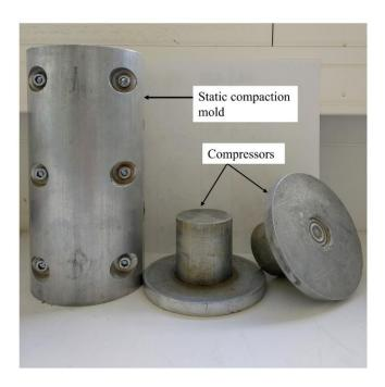
Fig. 2-3 Laboratory used Standard Static compaction tool.
