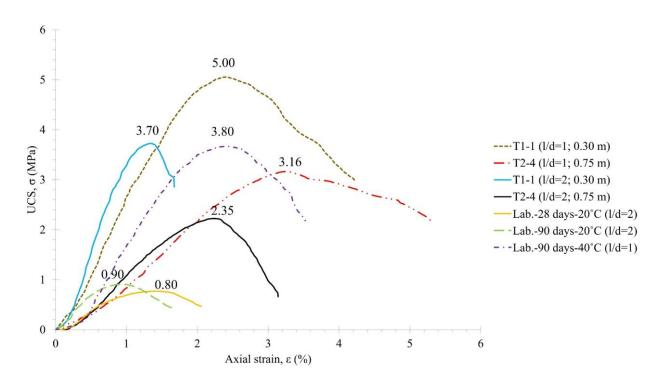
Fig. 3-4 UCS measured from the field- and laboratory-cured specimens.
