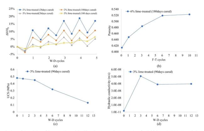
Fig. 1-6 Height variations of lime-treated materials subjected to 5 successive W-D cycles (after Cuisinier et al., 2014) (a), Evolution of porosity in lime-treated soil with respect to a number of F-T cycles (b) (Han et al., 2021), Evolution of UCS (c) and Hydraulic conductivity (d) in lime-treated soil subjected to 12 W-D cycles (Cuisinier et al., 2020).
