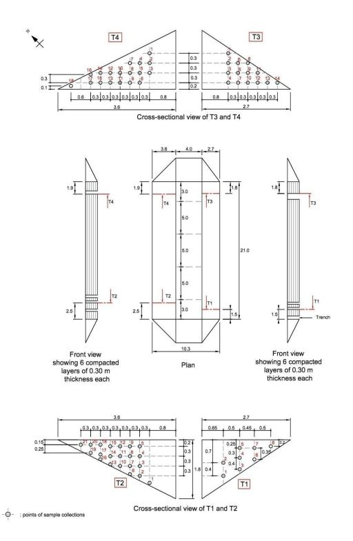
Fig. 3-3 Plan view, Front view along with Cross-sectional view of the excavated trenches made for sample collections from the lime-treated embankment (*All units in meter*)
