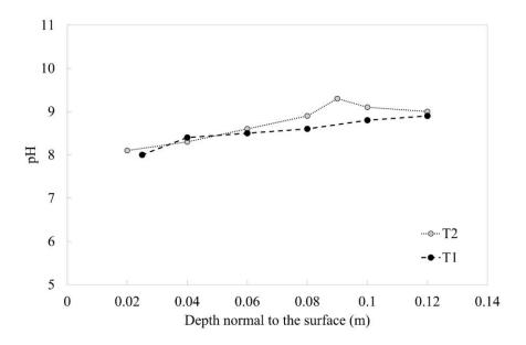
Fig. 3-9 pH measured on specimens sampled from the upper layer of the lime-treated embankment during deconstruction.
