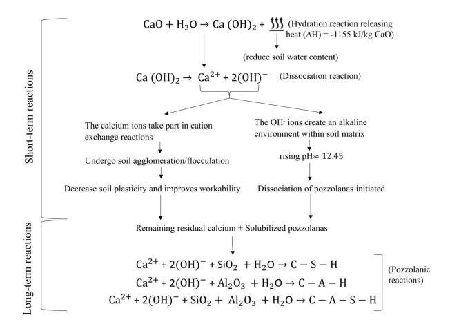
Fig. 1-2 Soil-lime physico-chemical reactions.
