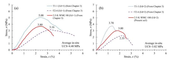
Fig. 4-10 Comparative evolution of UCS in in-situ core sampled and laboratory-accelerated cured soil of dimension of l/d ratio of 1 (a) and 2 (b).
