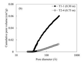
Fig. 3-12 Evolution of mesopores distribution (a) and cumulative pore volume (b) between T1-1 & T2-4 by BJH method.
