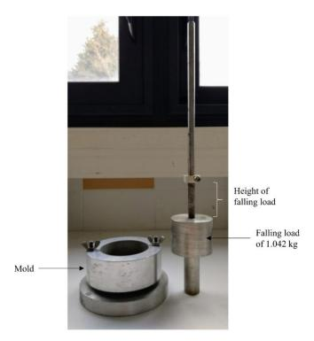
Fig. 2-2 Laboratory designed Mini Proctor compaction tool.
