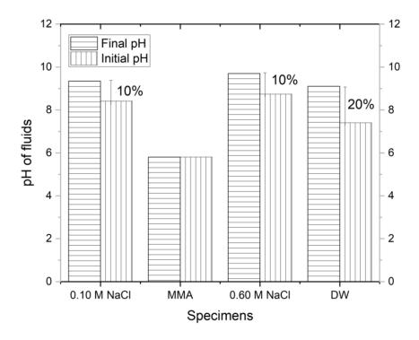
Fig. 7-4 Final pH measured in the effluents and compared with the initial pH of the respective fluids at the end of 5 W-D cycles.
