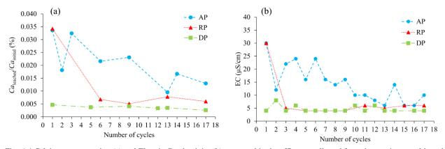
Fig. 6-4 Calcium concentration (a) and Electric Conductivity (b) measured in the effluents collected from the specimens subjected to W-D/D-W cycles as per AP, RP, and DP testing conditions.
