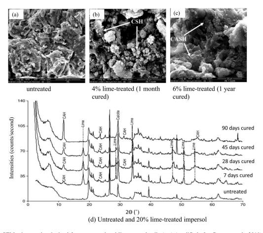
Fig. 1-4 SEM micrographs obtained from untreated and lime-treated soils (a-c) (modified after Rosone et al., 2019); (d) XRD pattern obtained from untreated and lime-treated impersol (d) (modified after Al-Mukhtar et al., 2010) subjected to different curing times.
