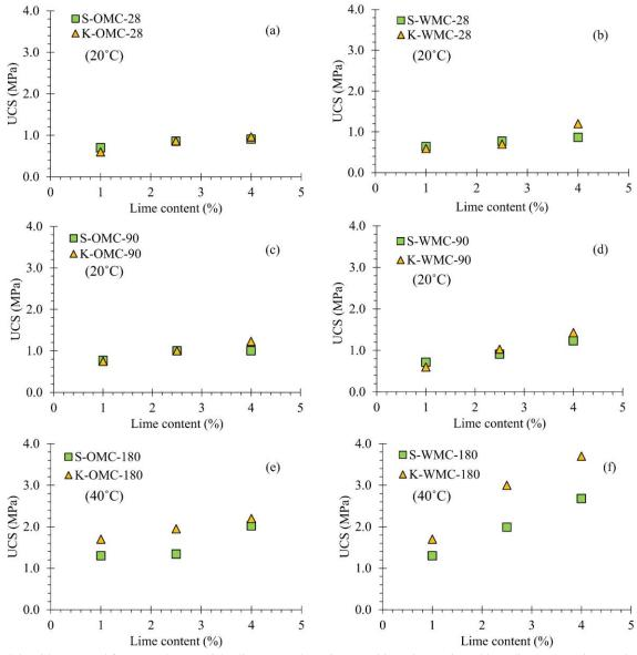
Fig. 4-2 UCS measured from 1%, 2.5% and 4% lime-treated specimens subjected to static and kneading compactions at OMC-28 days (a), WMC-28 days (b), OMC-90 days (c), WMC-90 days (d), OMC-180 days (e), and WMC-180 days (f).
