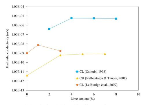
Fig. 1-9 Hydraulic conductivity evolution with respect to lime content.
