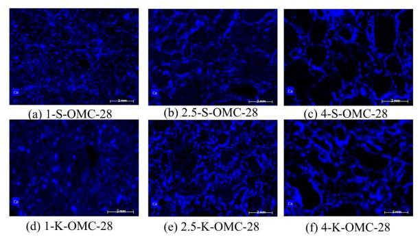
Fig. 4-7  $\mu$ -XRF image highlighting calcium distributions in 1%, 2.5%, and 4% lime-treated static (a, b, & c) and kneading compacted (d, e, & f) specimens prepared at OMC after 28 days of curing time at 20°C.
