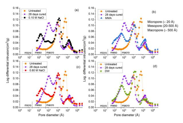
Fig. 7-5 Comparative evaluation of PSD in lime-treated specimens subjected to 0.10 M NaCl (a), MMA (b), 0.60 M NaCl (c), and DW (d) at the end of 5<sup>th</sup> W-D cycles with the with the untreated and the reference specimens by MIP.
