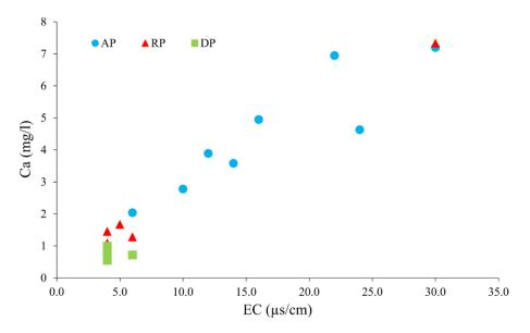
Fig. 6-6 Comparative evolution of calcium concentration and electric conductivity in the specimens subjected to W-D/D-W cycles.
