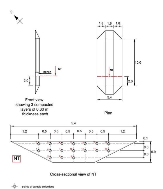
Fig. 3-2 Plan view, Front view along with Cross-sectional view of the excavated trench made for sample collections from the Untreated embankment (*All units in meter*)
