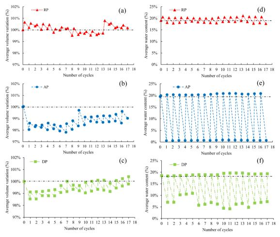
Fig. 6-2 Average volume variations (a-c), and water content variations (d-f) recorded from the specimens subjected to W-D/D-W cycles as per AP, RP, and DP testing conditions.
