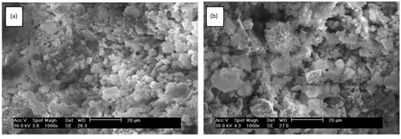
Fig. 1-12 SEM images of 5% hydrated lime-treated soil immediately after mixing (a), 48 hours after mixing (b) (modified after Di Sante et al., 2015).
