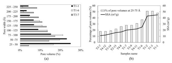
Fig. 3-14 Evolution of SSA with respect to the presence of pore volume in the mesopore range of pore diameter 25-75 Å.
