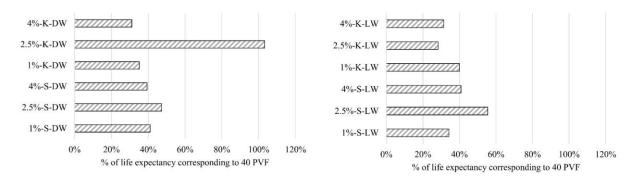
Fig. 5-5 Percentage of life expectancy that can be reached in a unit height earth structure if subjected to 40 PVF of DW (a) and LW (b) in kneading-and statically-compacted soil.
