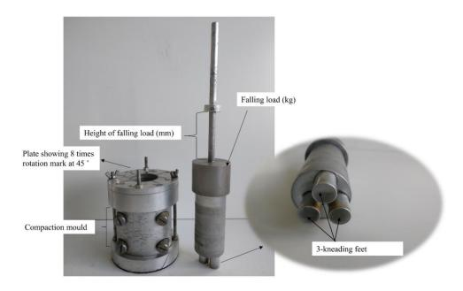
Fig. 2-4 Laboratory Kneading compaction tool.
