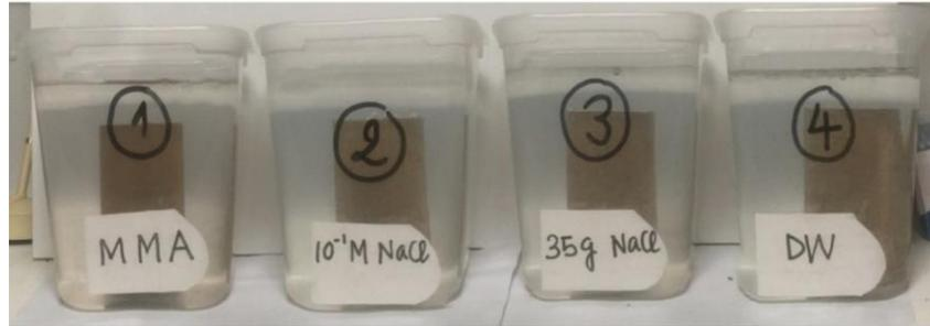
Fig. 7-1 Lime-treated specimens placed in four different fluids for 1<sup>st</sup> wetting during the W-D cycles.
