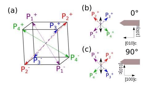
Figure 4.18: (a) Pseudocubic structure with the 8 possible directions of the polarization for BFO, 2 orientations are possible for the out-of-plane polarization and 4 for the in-plane polarization. Configuration of the tip and the up polarizations in the pseudocubic structure at (b) 0 ° and (c) 90°, the black arrow represents the lateral PFM signal.
