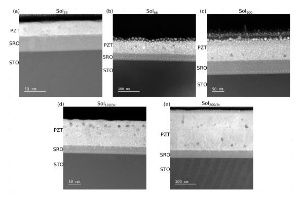
Figure E.2: (a) Original STEM images used for the study of cavities (a)  $sol_{33}$ , (b)  $sol_{66}$ , (c)  $sol_{100}$ , (d)  $sol_{100/3c}$  and (e)  $sol_{200}$
