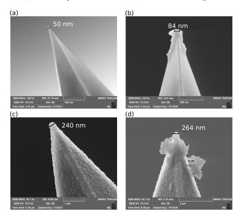
Figure 5.21: (a) New soft conductive tip and (b) the same kind of tip after usage. (c) New hard badly conductive tip and (d) the same kind of tip after mechanical switching experiments.
