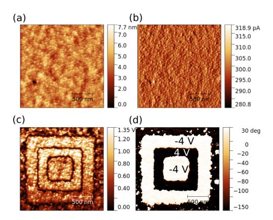
Figure 4.9: PFM images of the same region of the sol<sub>100</sub> sample. (a) Topography, (b) deflection (c) vertical amplitude, and (d) vertical phase. All images are  $2 \times 2 \mu m^2$  large.
