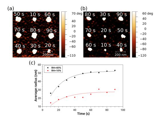
Figure 4.12: Phase PFM images of an experiment performed with a relative humidity (RH) of (a) 40% and (b) 10%. (c) Plot of the average equivalent radius measured vs duration of the voltage pulse for a RH of 40% and a RH of 10% with the fitting of Eq. 3.1
