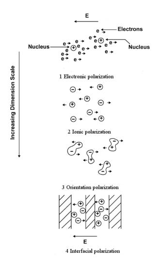
Figure 1.1: Different mechanisms of polarization (Dakin, 2006)
