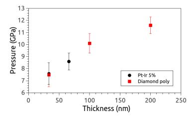
Figure 5.22: Plot of the pressure threshold against the thickness. The pressure threshold was obtained by applying Hertz's model to the results obtained in  $sol_{33}$ ,  $sol_{66}$ ,  $sol_{100}$  and  $sol_{200}$ .
