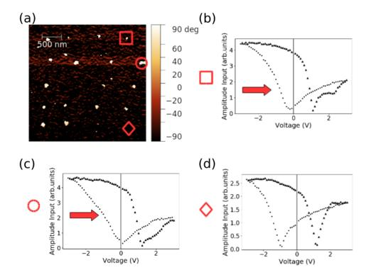
Figure 5.10: (a) Phase image of down domains created mechanically with 1.7  $\mu$ N in sol<sub>33</sub>, three points are marked by a square,a circle and a diamond. Amplitude off-field loops obtained while applying 1.7  $\mu$ N of (b) the square point, (c) the circle point and (d) the diamond point.
