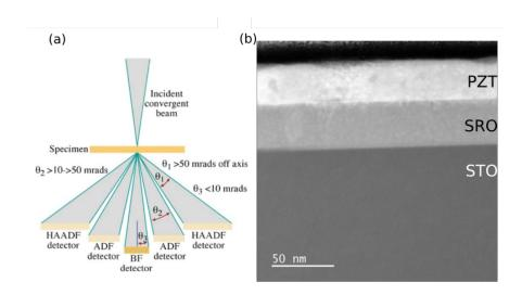
Figure 2.6: (a) Schematic of the beam geometry and the angular range for the different imaging modes in STEM where HAADF and bright field are shown (Williams and Carter, 2009). (b) HAADF imaging of one of the sol-gel-grown samples studied in this work, which consists of PZT over a SRO electrode and a STO substrate. The regions with higher Z atoms show higher intensity.
