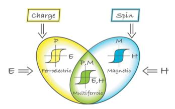
Figure 1.4: Ferroelectric/ferromagnetic multiferroic materials (Khomskii, 2009).
