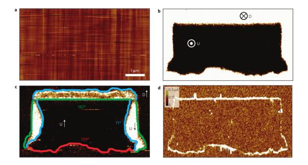
Figure 1.13: (a) Topography of a BFO sample (b) Vertical PFM of the same sample (c) Lateral PFM and the angle between domains d) Conductivity at domain walls. (Seidel et al., 2009)
