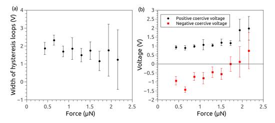
Figure 5.11: (a) Plot of the hysteresis loop width (the difference between positive and negative coercive voltage) against the force applied. (b) Plot of negative and positive coercive voltage against the force applied. All results obtained in sol<sub>33</sub> sample.
