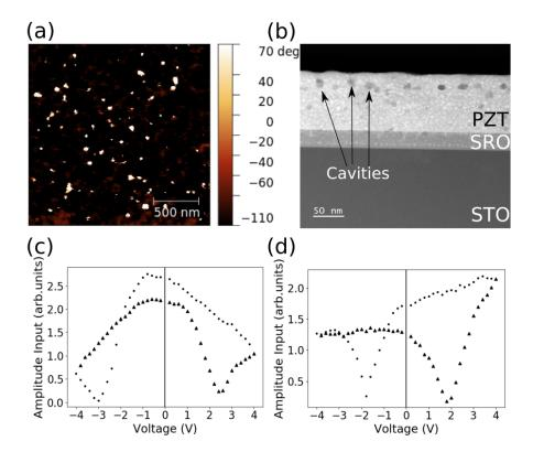
Figure 4.14: (a) Phase PFM image of the as-grown state of the  $sol_{100/3c}$  sample. (b) Cross-section STEM-HAADF image of the same sample as (a) where a line of cavities is visible close to the surface. (c) On-field loop where electrostatic effect are observed and (d) off-field loop in the same sample.
