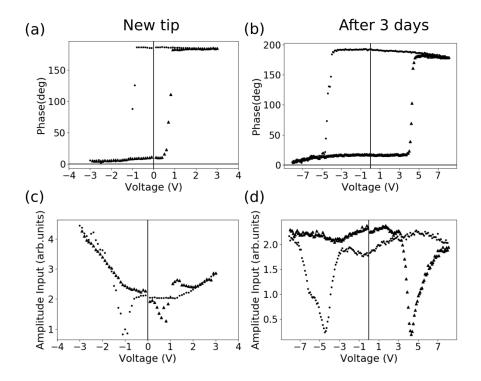
Figure 4.21: On-field (a) phase and (c) amplitude loops of BFO with a new tip. On-field (b) phase and (d) amplitude loops of BFO with a tip that has been used during three days.
