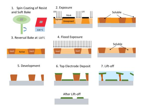
Figure 2.2: Reversal lift-off process (Liu, 2014)
