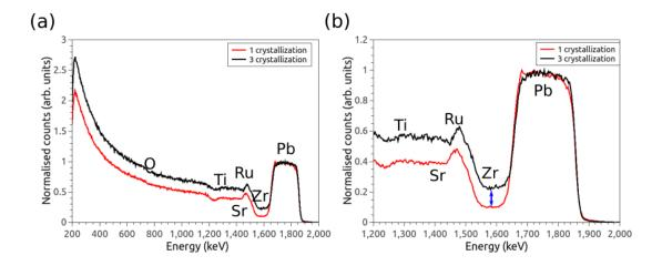
Figure 5.20: (a) RBS spectra and (b) peak of Pb for the  $sol_{100}$  and the  $sol_{100/3c}$  samples. A clear difference between both signals is present after the Pb peak (see blue arrow). This difference can be linked to porosity or roughness in the sample.
