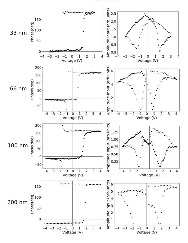
Figure 4.7: SS PFM on-field loops of phase and amplitude of the  $sol_{33}$ ,  $sol_{66}$ ,  $sol_{100}$  and  $sol_{200}$  samples. The ac voltage applied to the satellites to perform the PFM measurement was between 250 and 300 mV for all samples and the time steps in the range of a hundred ms.
