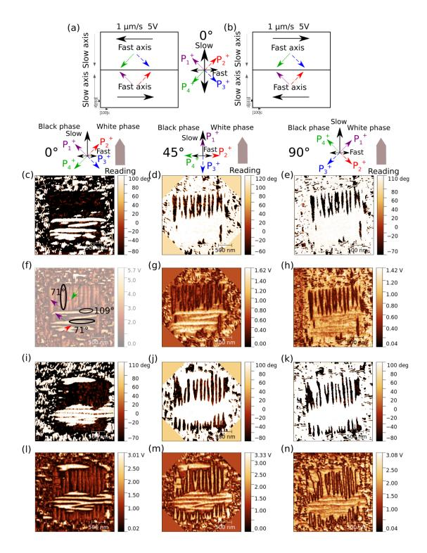
Figure 4.22: (a) Schematics for experiment 1 and (b) schematics for experiment 2 performed at 0° with the expected polarization. Lateral phase for experiment 1 at (c) 0°, (d) 45° and (e) 90°, and the corresponding amplitude images (f),(g) and (h). Lateral phase for experiment 2 at (i) 0°, (j) 45° and (k) 90°, and the corresponding amplitude images (l),(m) and (n). Image (f) also shows the different polarization directions and domain walls present in the experiment.
