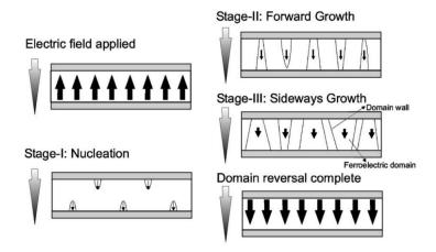
Figure 4.1: The three steps of ferroelectric switching when an electric field is applied (Dawber et al., 2005)
