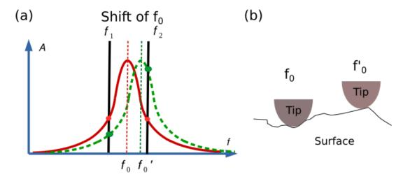
Figure 3.11: (a) Plot of two resonance amplitude peaks where the different frequencies and amplitudes involved in DFRT can be observed. When  $f_0$  shifts to  $f'_0$ ,  $A_1$  and  $A_2$  are not equal,  $f_1$  and  $f_2$  will change until their difference is null. (b) Schematic of a tip over the surface. Different contacts between sample and tip will create a change in the resonance frequency as the one shown in (a).
