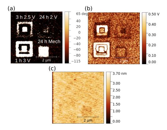
Figure 5.6: (a) Phase image of three patterns created electrically with  $\pm$  2,  $\pm$  2.5 and  $\pm$  3 V and a pattern switched mechanically. (b) Amplitude and (c) topography images of the same region. All images were obtained in the PLD<sub>20</sub> sample.
