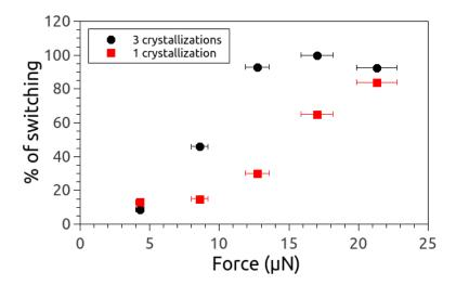
Figure 5.18: Plot of the percentage of switching against the force with a badly conductive tip for the  $sol_{100}$  and the  $sol_{100/3c}$  samples.
