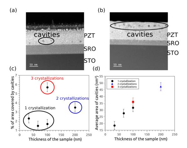
Figure 5.19: STEM-HAADF images of (a)  $sol_{100}$  and (b)  $sol_{100/3c}$  with visible cavities. Plot of (c) percentage of area covered by cavities and (d) average area of cavities against the thickness of the sample.
