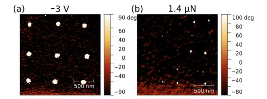
Figure 5.5: (a) Phase image of a region with 9 points switched by -3 V applied for 10 to 90 seconds (b) Phase image of a region where 1.4  $\mu$ N were applied during 60 seconds in 25 points, not all points switched. Both images were obtained in sol<sub>33</sub>.
