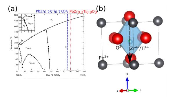
Figure 1.15: (a) Phase diagram of the transition temperature and structure of PZT (Jaffe et al., 1971) and (b) sketch of the tetragonal structure of Pb[Zr<sub>0.2</sub>Ti<sub>0.8</sub>]O<sub>3</sub>, the black arrow indicates the direction of the ferroelectric polarization.
