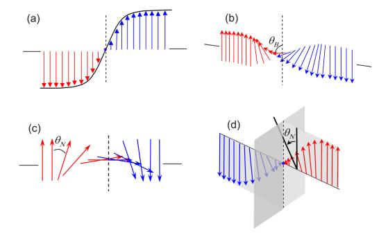
Figure 1.10: Different types of domain walls (a) Ising (b) Bloch (c) Néel d) Mixing Ising-Néel. (Lee et al., 2009).
