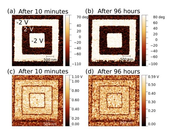
Figure 4.11: PFM images of the same region of a 33 nm thick PZT sol-gel film. (a) and (c) vertical amplitude and phase image of a pattern created with 2 V and -2 V after 10 minutes. (b) and (d) vertical amplitude and phase image of the same pattern after 96 hours.
