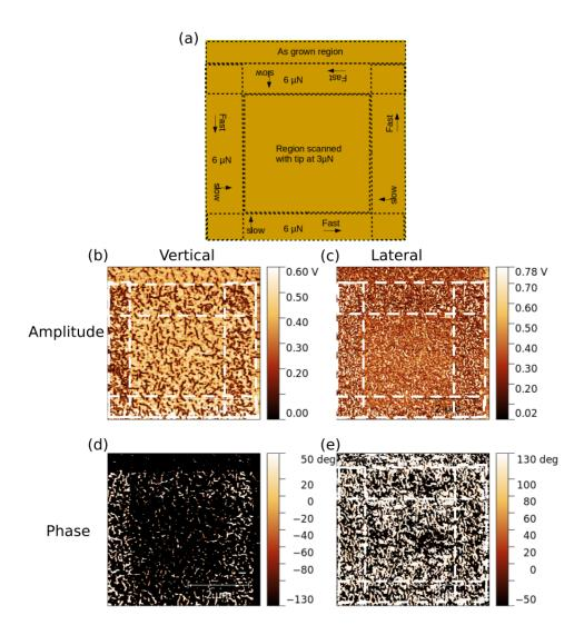
Figure 5.23: (a) schematic of force applied in the sample and their direction. (b) Vertical and (c) lateral PFM amplitude images. (d) Vertical and (e) lateral PFM phase images.
