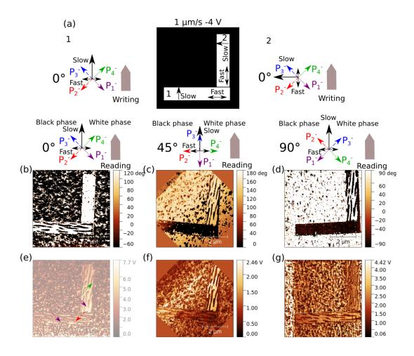
Figure 4.25: (a) Schematics for experiment 1 and 2 performed at 0° with the expected polarization. Lateral phase at (b) 0°, (c) 45° and (d) 90°, and the corresponding amplitude images (e),(f) and (g). Image (e) also shows the different polarization directions present in the experiment.
