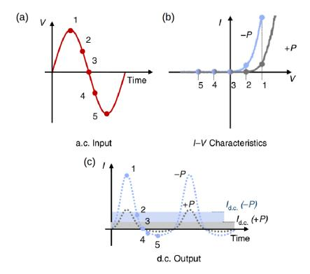
Figure 1.14: (a) AC input in a domain wall in ErMnO<sub>3</sub> (b) I-V curve of the domain wall for both polarizations (c) Final output of the domain wall for both polarizations where the signal is half wave rectified(Schaab et al., 2018).
