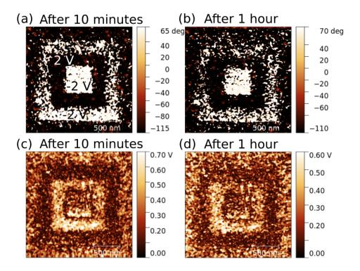
Figure 4.16: (a) and (c) vertical amplitude and phase image of a pattern created with 2 V and -2 V in the  $PLD_{20}$  after 10 minutes. (b) and (d) vertical amplitude and phase image of the same pattern after 1 hour.
