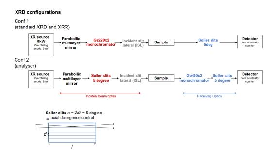
Figure B.1: Configuration 1 (Conf 1) and configuration 2 (Conf 2) used for the x-ray reflectometry and diffraction experiments.
