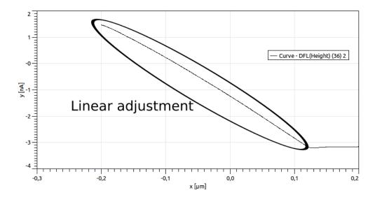
Figure 5.4: Force curve of the setpoint (y) against the displacement (x).
