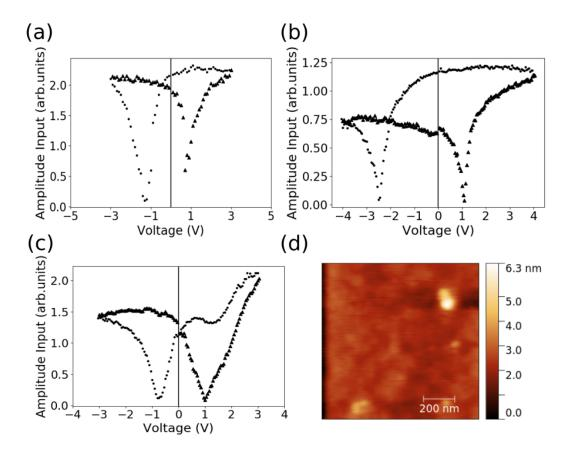
Figure 4.17: Off-field loops for the (a) PLD<sub>20</sub> and the (b) PLD<sub>40</sub> sample. (c) on-field loop of the 40 nm sample showing a deformation related with the growth of a hillock. (d) topo of the 40 nm sample with a hillock on it.
