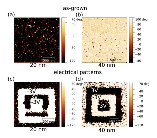
Figure 4.15: Phase PFM image of the as-grown state of the (a)  $PLD_{20}$  and the (b)  $PLD_{40}$  samples. Phase PFM image of patterns created with 3 V and -3 V in the (c)  $PLD_{20}$  and the (d)  $PLD_{40}$  samples.
