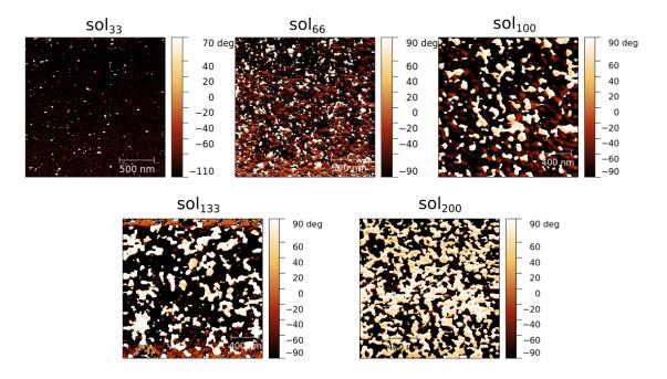
Figure 4.4: PFM phase images of the  $sol_{33}$ ,  $sol_{66}$ ,  $sol_{100}$ ,  $sol_{133}$  and  $sol_{200}$  samples. The images are  $2 \times 2 \mu m^2$  large and the scale at the bottom right represents 400 nm. In these images, the down polarization is represented in white, while the up polarization is represented in dark.
