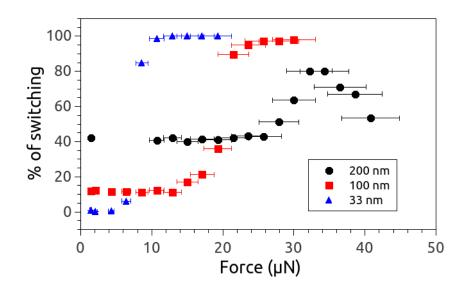
Figure 5.15: Plot of the percentage of switching against the force with a badly conductive tip for the  $sol_{33}$ ,  $sol_{100}$  and  $sol_{200}$  samples.
