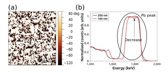
Figure 4.13: (a) Phase PFM image of the as-grown state of the  $sol_{166}$  sample. (b) RBS spectrum around the Pb peak for the  $sol_{200}$  and the  $sol_{166}$ . The arrow indicates the decrease of Pb signal for the  $sol_{166}$ , which can be related to a different composition in the middle of the sample. The peak width is related to the thickness of PZT.
