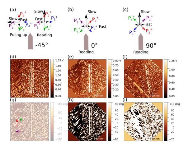
Figure 4.23: (a) Schematics of the tip and polarization for the (a) -45°, (b) 0° and (c) 90°. Lateral amplitude image of the sample at (d) -45°, (e) 0° and (f) 90°. Lateral phase image of the sample at (g) 45°, (h) 0° and (i) 90°. (g) Shows the different polarization directions present in the experiment.
