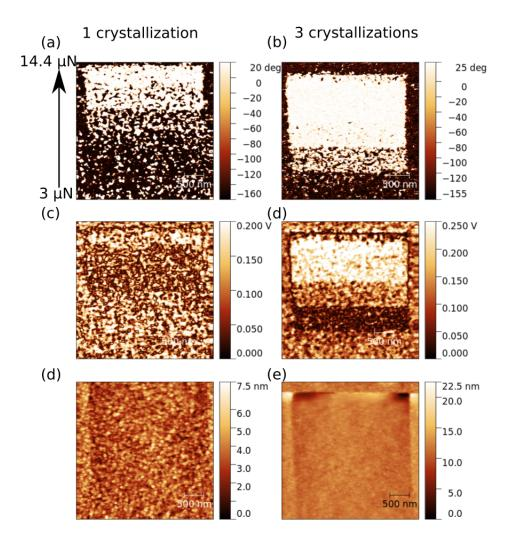
Figure 5.17: Mechanical switching for the  $sol_{100}$  sample and the  $sol_{100/3c}$  sample. (a) and (b) PFM phase images, (c) and (a) PFM amplitude image, and (d) and (e) topography.
