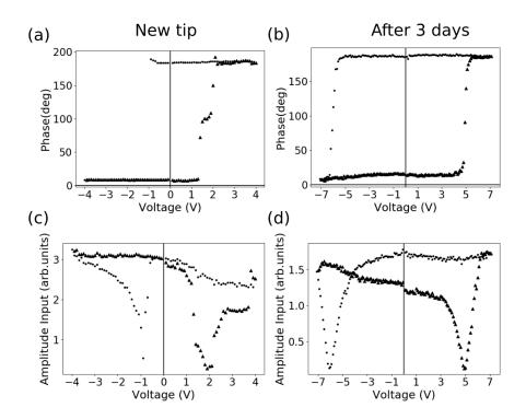
Figure 4.20: Off-field (a) phase and (c) amplitude loops of BFO with a new tip. Off-field (b) phase and (d) amplitude loops of BFO with a tip that has been used during three days.
