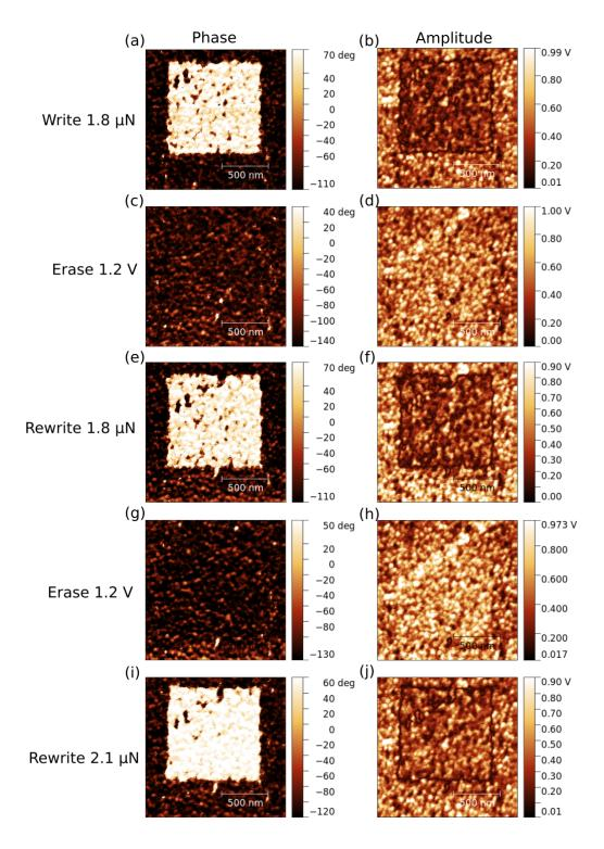
Figure 5.13: PFM phase and amplitude images after (a) and (b) writing mechanically in an as-grown region with 1.8  $\mu$ N, (c) and (d) erasing electrically the domain mechanically written with 1.2 V, (e) and (f) rewriting the same region with 1.8  $\mu$ N, (g) and (h) erasing again with 1.2 V, and (i) and (j) rewriting with 2.1  $\mu$ N to see if it was possible to switch the unswitched regions with 1.8  $\mu$ N.
