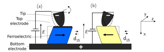
Figure 3.8: Schematics for lateral PFM. Like in vertical PFM, different directions of the polarization create different deformations in the material. (Brugère, 2011)
