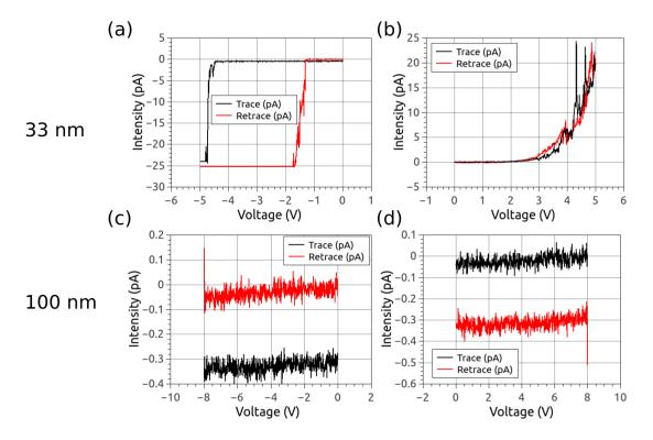
Figure 4.8: C-AFM I-V curves for the  $sol_{33}$  (a) and (b), and for the  $sol_{100}$  (c) and (d). The voltage ramps were performed at 0.5 V/s. The black lines represent the voltage going to 0 to the extreme (positive or negative), while the red lines represent the voltage going back to 0.
