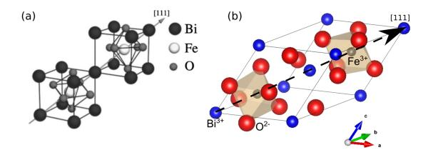
Figure 1.16: (a) Pseudocubic structure (Ederer and Spaldin, 2005) and (b) sketch of the rhombohedral structure of BiFeO<sub>3</sub>, the black arrow indicates the direction of the ferroelectric polarization.
