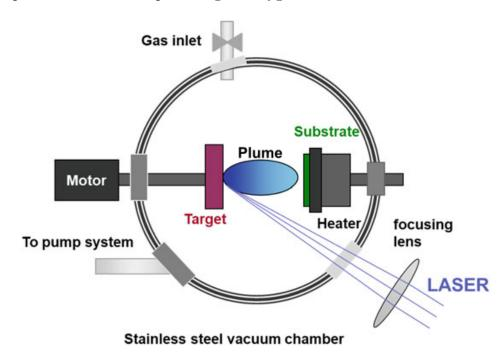
Figure 2.4: Schematics of PLD system (Craciun et al., 2020).
