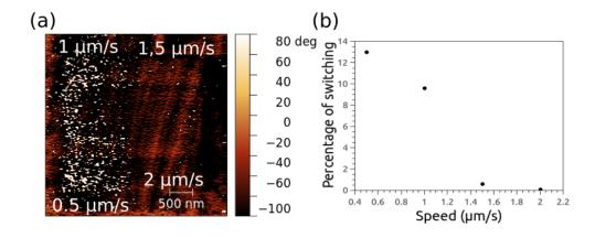
Figure 5.7: (a) Phase image of the four regions mechanically switched with different speeds. (b) Plot of the percentage of switching against the scanning speed. The experiment was performed in sol<sub>33</sub> sample.
