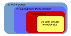
Figure 1.5: All ferroelectric materials are piezo and pyroelectrics.
