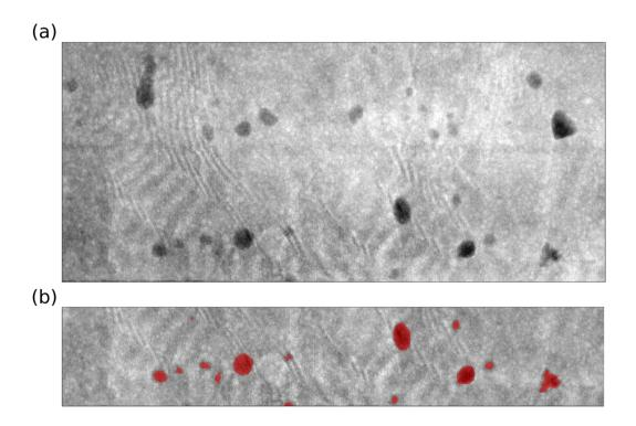
Figure E.1: (a) Original STEM image of the  $sol_{200}$  samples. (b) Bottom part of the image cut for image processing. The regions in red have been selected by the software as cavities.
