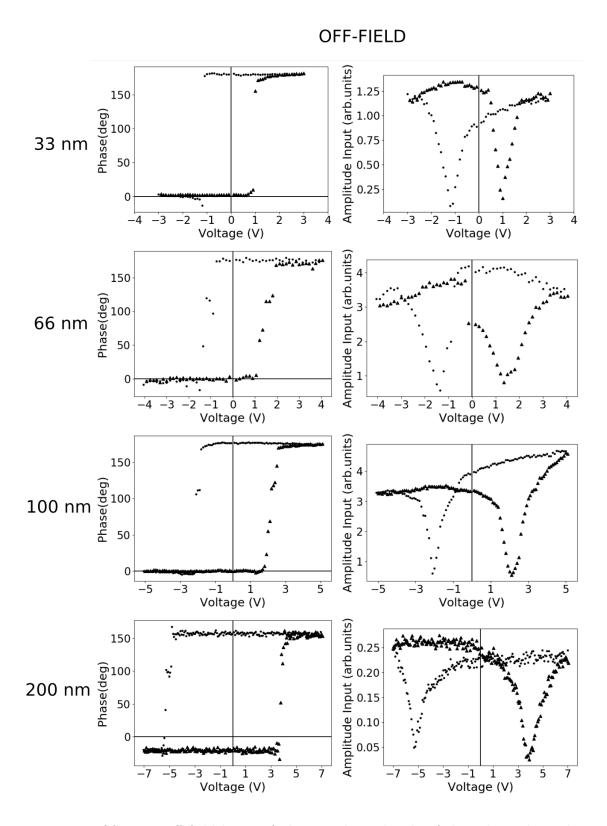
Figure 4.6: SS PFM off-field loops of phase and amplitude of the  $sol_{33}$ ,  $sol_{66}$ ,  $sol_{100}$  and  $sol_{200}$  samples. The ac voltage applied to the satellites to perform the PFM measurement was between 250 and 300 mV for all samples and the time steps in the range of a hundred ms.
