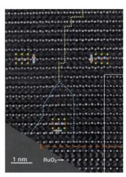
Figure 1.7: On the left, schematic of two domains separated by a domain wall (in blue). On the right, high-resolution transmission electron microscope image at the atomic scale of three domains and their domain walls in Pb[Zr<sub>0.2</sub>Ti<sub>0.8</sub>]O<sub>3</sub>, domain walls are represented by the dotted line (Jia et al., 2011).
