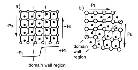
Figure 1.11: (a) 180° domain wall, the position of the middle atom gives the polarization in the region (b) 90° degrees domain wall (Damjanovic, 1998).
