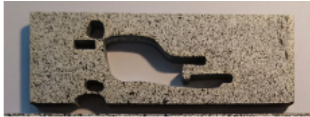
Figure 6.7: Example of an optimized sample geometry manufactured in fir wood with a black and white paint speckle pattern, figure from [Chamoin et al. , 2020].
