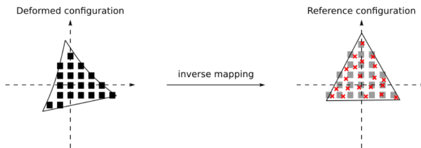
Figure 6.15: Schematic of the deformation procedure of a synthetic image for one triangular element. The black squares depict the pixels positions in the deformed configuration, while the grey squares depict the pixels positions in the reference one. The red crosses denote the pixels from the deformed configuration projected by an inverse mapping in the reference one. The deformed image for the element is obtained by interpolating the grey levels from the grey squares onto the crosses.
