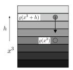
Figure 1.8: Fluid parcel in a stratified environment
