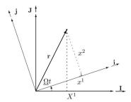
Figure 1.3: Inertial framework versus rotating framework
