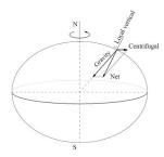
Figure 1.4: The effects of the centrifugal force
