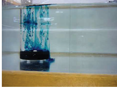
Figure 1.7: Side view of a Taylor columns experiment
