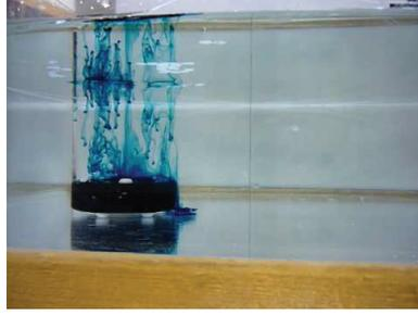
Figure 1.7: Side view of a Taylor columns experiment
