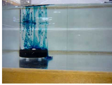
Figure 1.7: Side view of a Taylor columns experiment
