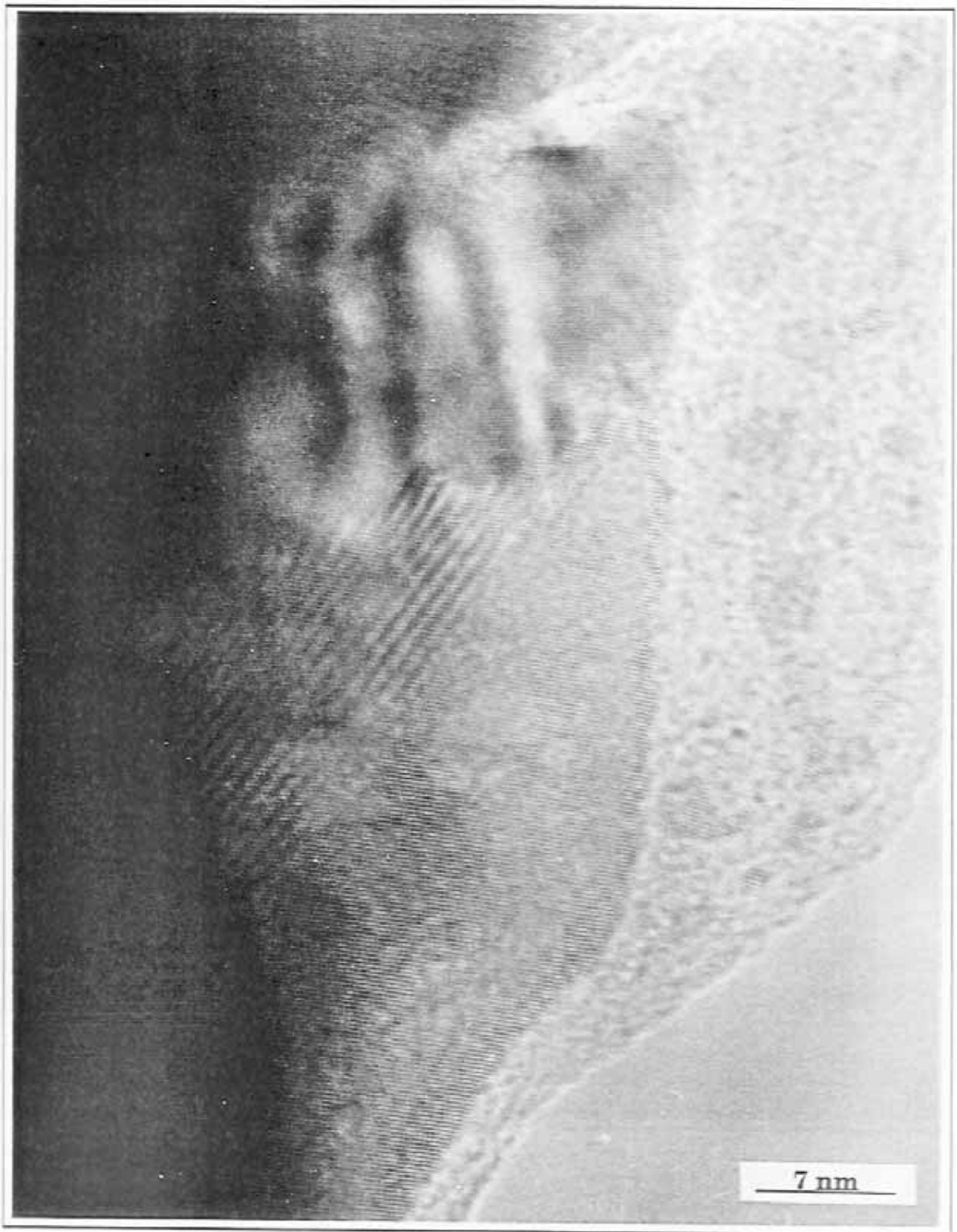
Figure 13 : HRTEM image of the particular phase present in layer 2 prior to matrix infiltration.
