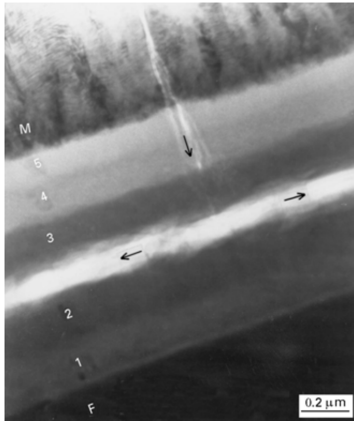
Figure 4 : Bright-field image of matrix crack deflection (arrows) in compositional gradient interphase A'. (F: fibre; M: matrix; the numbers relate to the five different sublayers involved in the interphase.)
