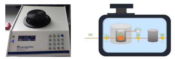
Figure 34. A photo (left) and a schematic diagram (right) of the AccuPyc II 1340 pycnometer; a, b and c are the valves.<sup>129</sup>
