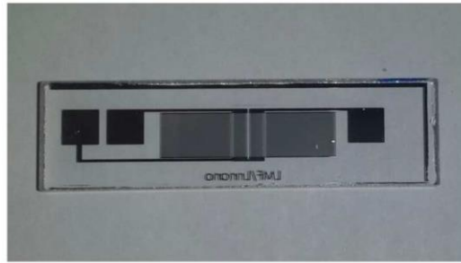
Figure 1-32 Dispositif SAW sur quartz (Della Lucia et al. 2015)
