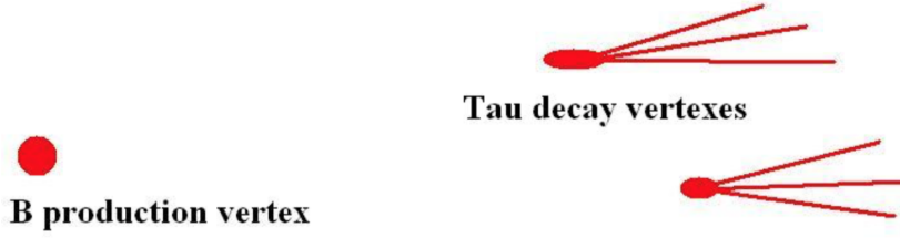
Figure 5.4: Schematic view of a B_{(s)}^0 \rightarrow \tau^+(\rightarrow 3\pi^\pm\nu_\tau)\tau^-(\rightarrow 3\pi^\pm\nu_\tau) decay in the LHCb detector. Courtesy of A. Morda [139].
