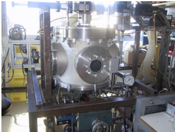
Figure II-3-a : Installation plasma sous vide IFTH [IFTH 2008]
