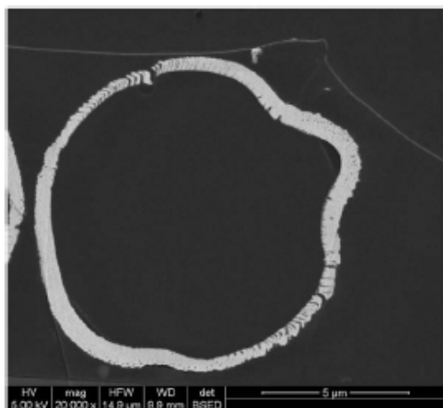
Fig. 2. SEM images (BSE) of cross polished sections of HF-27 wt.% Ta deposit on carbon fiber tested at temperature 1850 °C under high vacuum during 5 s.
