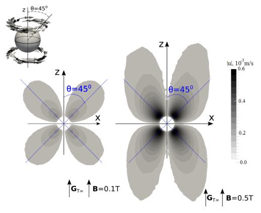
**Figure 3.8:** Effect of the intensity of the magnetic field **B** on the flow around the spherical particle, the case of the vector **B** parallel to the imposed thermal gradient  $\mathbf{G}_{T,\infty}$  is considered, from the ref. [50]
