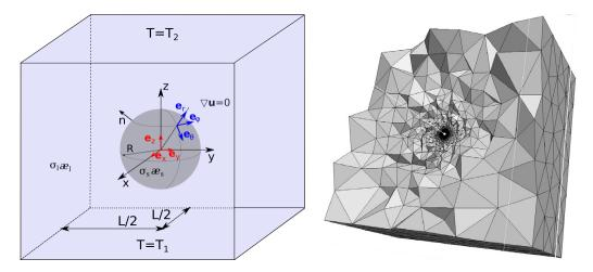
*Figure 3.6:* Configuration of a calculation domain for the numerical simulations (a) and illustration of the mesh used for calculations to capture the strong variations of the physical variables near the surface of the particle, from the ref. [50]
