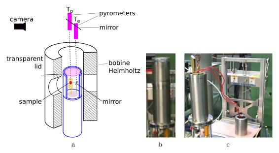
**Figure 4.9:** Scheme of the AEXAM set-up, first version: a) Complete installation with the Helmholtz coil providing DC magnetic field up to 5 T directed horizontally and the double-wall water cooled vacuum chamber inserted in the coil; b) Photo of the vacuum chamber which consisted of 2 parts and c) Photo of the opened vacuum chamber to show the ELM inductor, mirror and tubes for water cooling
