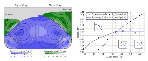
Figure 4.3: a) Illustration to the effect of the amount of glass charged in the crucible on the height of the dome of the metal and of the glass; b) Comparison of the results of solution of eqs.(4.1)-(4.4) and results obtained numerically for the height of the metal and the glass for different amount of the latter,  $B_0 = 0.13$  T, the vertical lines indicate the transition between different surface geometry as shown in inserts, from ref. [58]
