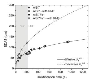
**Figure 2.1:** Secondary dendrite arm spacing (SDAS) on solidification time for Al-7wt%Si and Al-7wt%Si7-1wt%Fe alloys processed under diffusive conditions (filled symbols) and forced fluid flow (RMF; open symbols) with Solidification and Quench Furnace (circles, grey shaded region) and Low Gradient Furnace (diamonds)[6]
