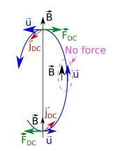
**Figure 1.1:** Damping effect expected with use of the DC magnetic field: the induced electromagnetic force is directed opposite to the velocity of the liquid
