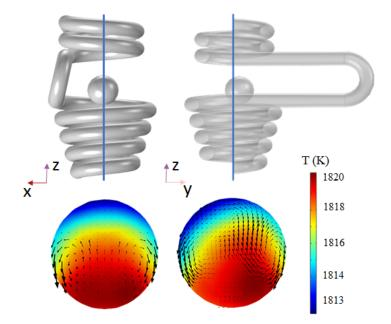
*Figure 5.2:* Effect of the geometry of the indctor on the flow in a levitating droplet studied with  $\text{COMSOL}^{\textcircled{R}}$  Multiphyscis R, sample deformation is not taken into account, by R. Pons at el., submitted to Magnetohydrodynamics
