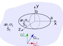
Figure 3.4: Particle in the form of prolate spheroid (ellipsoid) in the infinite liquid pool under the external thermal gradient  $\mathbf{G}_{T,\infty} = \mathbf{e}_x G_{T,\infty}^{\parallel} + \mathbf{e}_y G_{T,\infty}^{\perp}$
