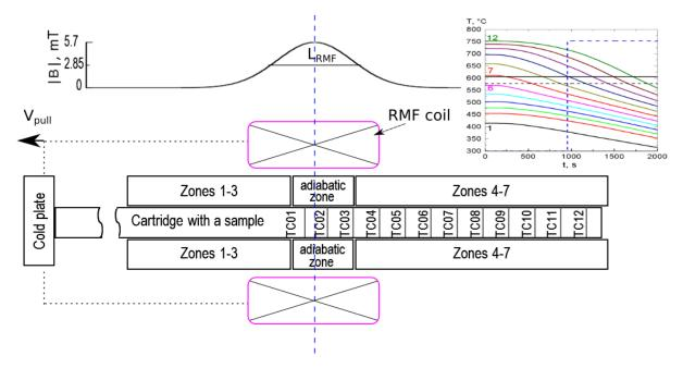
**Figure 2.4:** Scheme for the experimental set-up used in solidification experiment in microgravity with indication of the positions of thermocouples and example of obtained temperature curves, the intensity of the effective value of magnetic field along the growth direction is shown at the top part of the drawing [8]
