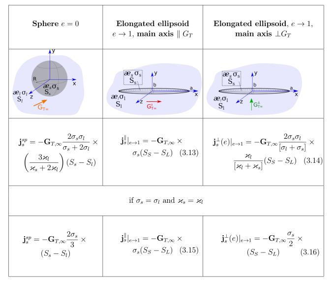
Table 3.1: Comparison of the thermoelectric current originated in a spherical particle and in a highly elongated ellipsoid for two different orientation of the latter with respect to the thermal gradient
