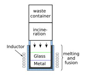
Figure 4.1: Scheme of the PIVIC process
