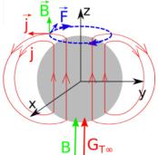
**Figure 3.7:** Illustration for the thermoelectric current in the liquid and appearance of the azimuthal magneto-thermoelectric force, case of a spherical particle and vec-) tors  $\mathbf{B}$  and  $\mathbf{G}_T$  co-directed along the z-axis
