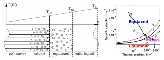
Figure 2.9: a)Presentation of the columnar and equiaxed zone:  $T_L$  - liquidus temperature of the alloy,  $T_{ne} < T_l$  - temperature of nuclei formation,  $T_{CF} < T_{ne}$  - temperature at the tip of columnar dendrites, which can be below the  $T_{ne}$  because of kinetics effect, from ref. [16], b) Hunt diagram calculated for the refined Al-7wt%Si alloy, zones of different growth are indicated, from ref. [17]
