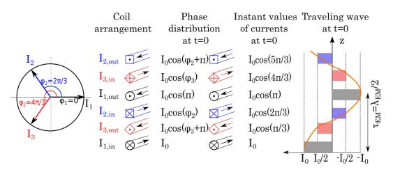
**Figure 1.4:** Illustration to the current supply in a three-phase linear motor: the 3 AC currents circulate in the system with phase difference of  $2\pi/3 = 120^{\circ}$ , but due to the coils' arrangement the phase shift between neighboring coils is  $\pi/3$ . Attention should be given to the actual current direction: the "out" direction with the phase ( $\varphi_3 + \pi$ ) corresponds finally to the direction "in".
