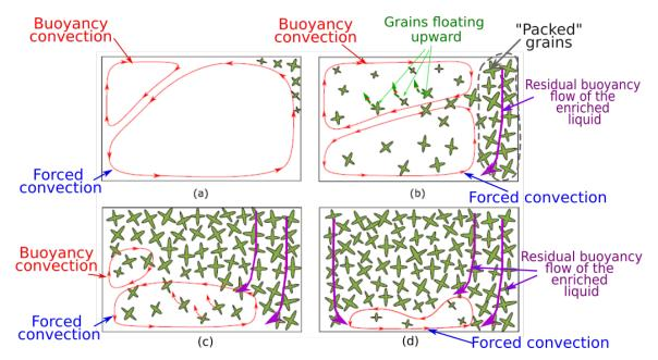
*Figure 2.12:* Illustration to the effect of the buoyancy and forced convection during the solidification process, from the PhD Thesis of Tao Wang [26]
