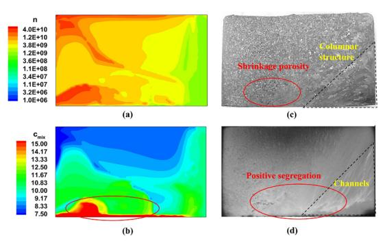
**Figure 2.13:** Comparison of numerical simulations and experimental observations: calculated grain number density distribution (a), calculated macrosegregation map at center plane of the sample (b), grain structure of ingot(c) and X-radiography of the ingot (d), the figure is taken from the ref. [27]
