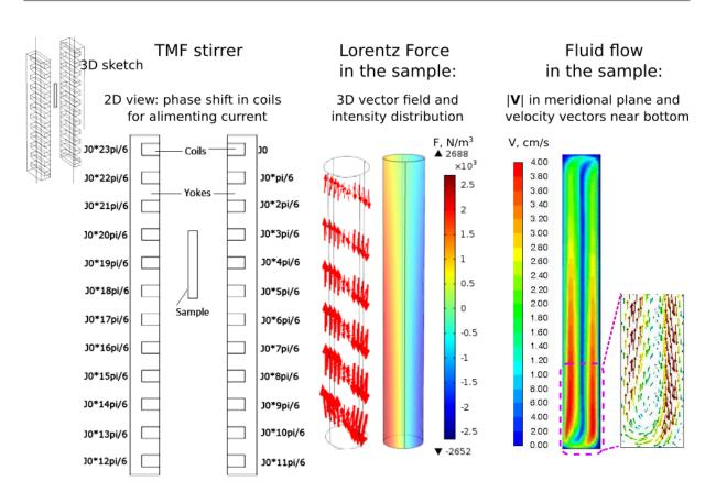
**Figure 2.7:** Scheme of TMF stirrer developed in the Materials Science Research group of University of Miskolc, Lorentz force in the sample calculated with  $\text{COMSOL}^{\textcircled{R}}$  Multiphysics R software and fluid flow obtained in crucible filled with the melt under the action of calculated force taken with the factor 0.1 and gravity, the figures are taken from the ref. [13]
