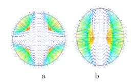
**Figure 4.6:** Electromagnetic force acting on the droplet with the AC current having: opposite phases in the top and bottom coil, quadruple filed (a) and the same phase on the coil, bipolar field (b)
