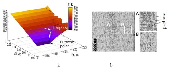
**Figure 2.3:** a) Liquidus plane for AlSiFe alloy in Al-rich corner, interpolated with data obtained from CIRIMAT (J.Lacaze, private communication); b) Image of the sample showing segregation of Si and accumulation of  $\beta$ -phase in the sample center
