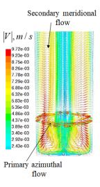
Figure 2.5: Scheme of the flow under the effect of RMF in microgravity experiments, from presentation at SP17 conference
