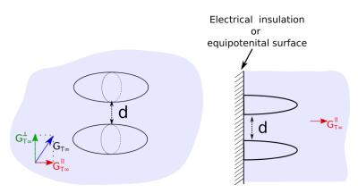
**Figure 5.1:** Example of configurations for the theoretical study of the thermoelectric problems: first step toward the effect of particles' interaction on the thermoelectric current
