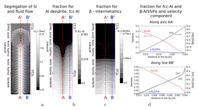
**Figure 2.6:** Results of simulations: a)Segregation pattern for Si and superposed flow field; b)Distribution of the volume fraction of Al-rich dendrites; c)Distribution of the volume fraction of  $\beta$ -intermetallics; d)Distribution of volume fractions of the two solid phases and module of the axial and radial velocities along the lines indicated in figs.a-c, from [8]
