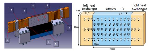
**Figure 2.10:** Scheme of the AFRODITE facility and sketch showing the positions of the thermocouples on the side wall of the crucible. Indicated components of shown AFRODITE setup : (1) sample, (2) left heat exchanger, (3) resistance, (4) stainless steel crucible, (5) thermocouples positions, (6) right heat exchanger, (7) water cooling system, (8) flat electromagnetic inductor, the figures are taken from the ref. [22]
