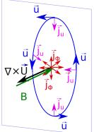
**Figure 1.2:** Cancelling of the eddy current when DC magnetic field is directed parallel to the vorticity of the flow: $j_{Phi} \approx \sigma \nabla \Phi$  cancels  $j_u \approx \sigma u B$
