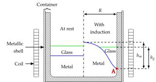
**Figure 4.2:** A meridional section of the melter, the metal is covered with the glass: the deformation of the surface of the metal due to the electromagnetic pressure, and the formation of a dome emerging from the glass is shown on the right, this figure corresponds to the Fig.2 from the ref.[58]
