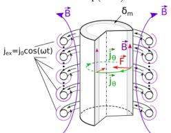
**Figure 1.3:** With use of the monophase AC current in the coil: magnetic fields penetrates in the load over the distance  $\delta_m$  (eq.(1.11)), the eddy current is mainly generated there. The averaged in time Lorentz force is directed perpendicularly to the surface of the load and plays the role of a magnetic pressure.
