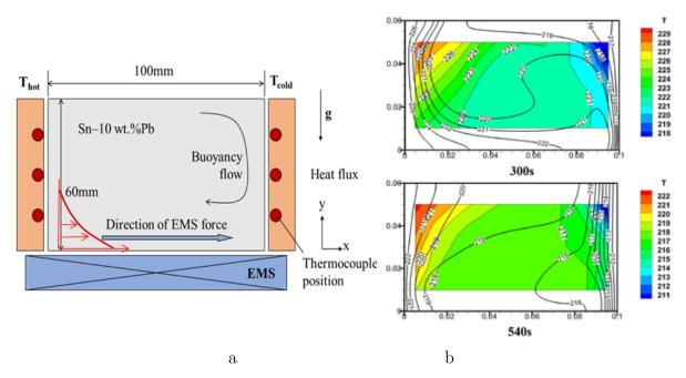
**Figure 2.11:** a) Scheme presenting flow directions in the experiment and b) Comparison of temperature obtained in simulations with  $A_{emf} = 180N/m^3$  and measured during the experiment: two-dimensional temperature field in the beginning (upper figure, t=300s) and in the middle (t=540s, lower figure) of solidification process, from [27]
