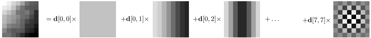
Figure 1.5: Decomposition of a 8 \times 8 spatial image into a linear combination of 64 DCT filters.
