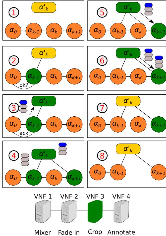
Figure 3.4: Steps to achieve migration. Each  $\alpha_k$  is a Virtual Network Function in the chain. There is an exchange of messages among orchestrators of the Virtual Network Functions to coordinate the migration.
