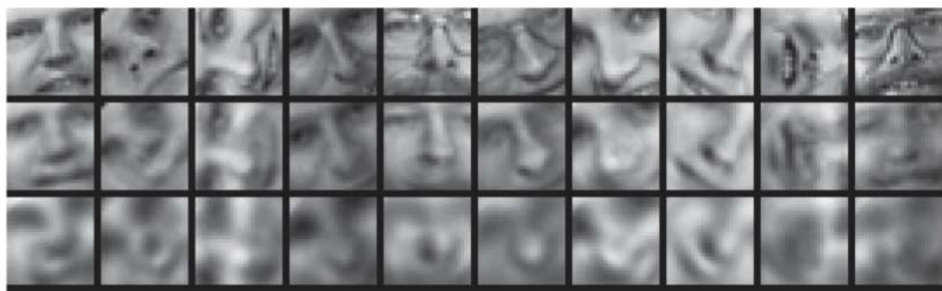
Figure 2.6: Top to bottom: A random test image from each class; reconstructions by the 30-dimensional autoencoder; reconstructions by 30-dimensional standard PCA. (taken from [Hinton and Salakhutdinov, 2006]).
