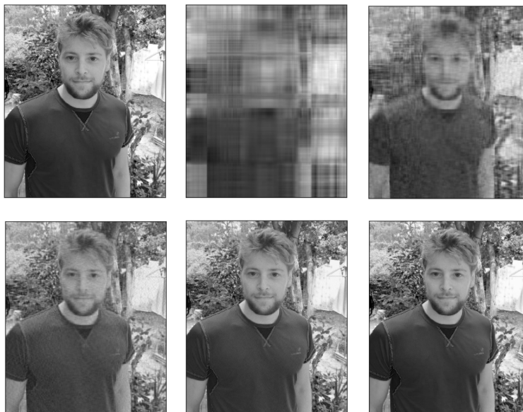
Figure 2.1: Original image and the following SVD approximations of rank 5, 20, 63, 191 and 446.
