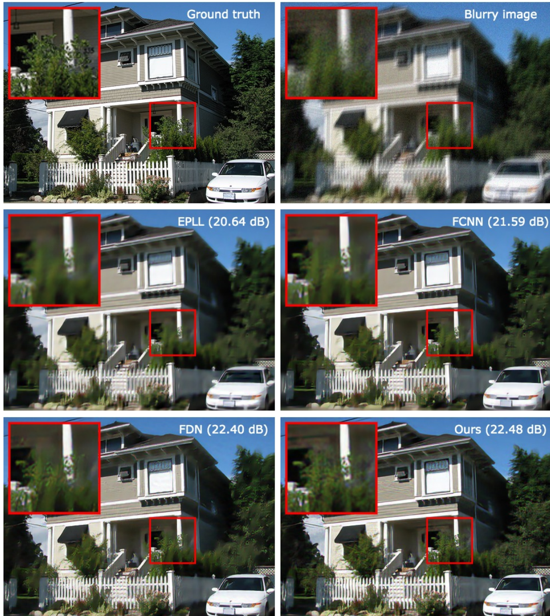
Figure 4-7: Example of image deblurring with an additive noise of 3% (better seen on a computer screen). In this example, we obtain better PSNR scores than competitors and better visual results, for example details around the door or the leaves.
