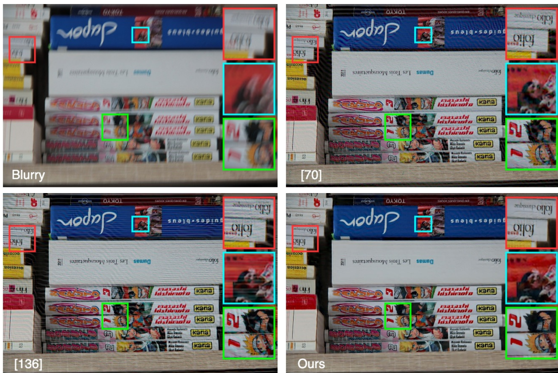
Figure 4-11: Real-world blurry images deblurred with camera shake estimated with the approach of Whyte et al. [126]. The proposed approach restores sharp edges next to the books cover without introducing ringing artifact nor amplifying the noise.
