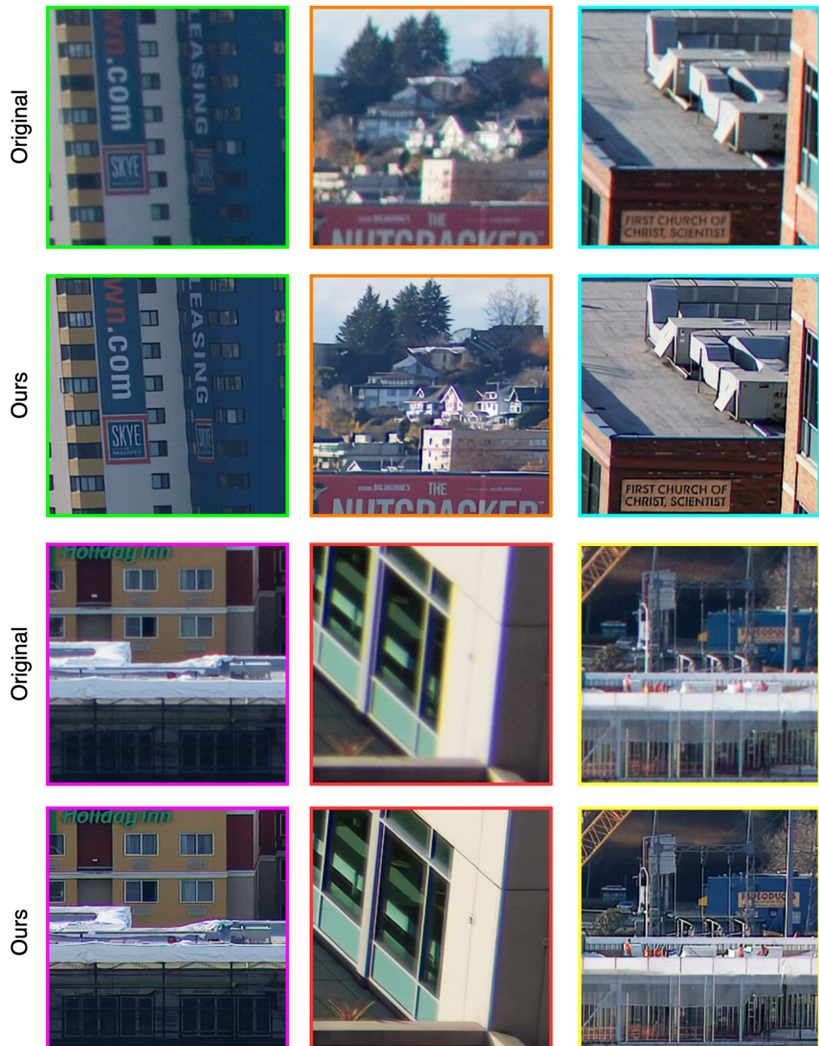
Figure 5-8: Comparisons between the original image and our restored version of the image shown in Figure 5-7. For instance the trees in the orange box or the building in the red box exhibit chromatic aberrations and the panels in the green box and the cyan box are blurred by the monochromatic aberrations. Our method removes these corruptions, resulting in a sharper image (better seen on a computer screen).
