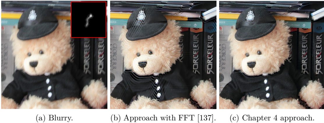
Figure 1-3: The teddy bear image is blurry because of camera motion during exposure. The blur has been estimated beforehand with a blur estimation method and is shown in the red box (it is zoomed by a factor 3). The deconvolution approach based on FFT introduces artifacts around the badge on the hat and next to the buttons and collar. The proposed approach in Chapter 4 also removes the blur without producing these artifacts. The full image is shown in Chapter 4 addressing motion blur.
