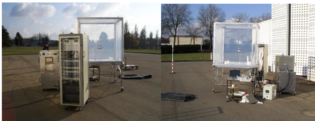
Figure 2-8: The 3.4 m 3 moveable simulation chamber in ICARE, Orleans, France
