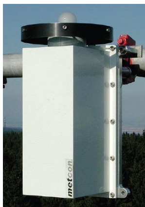
Figure 2-30: Diode Array Spectrograph with actinic optics
