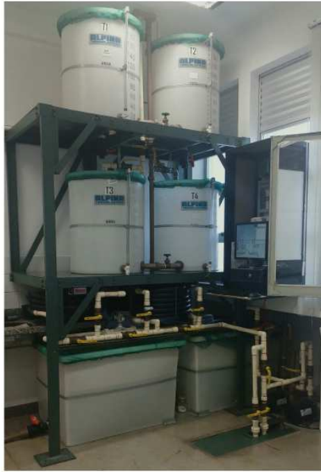
Figure 2.3: Interactive Tank System used in the experiments available at the CEFET-MG, Divinópolis, Brazil.
