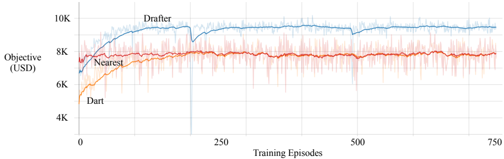
Figure 3.10: Training curves for the Dart (orange) and Drafter (blue) agents over 750 instances of size 1400/14. Nearest (red) is provided as a reference. Darker curves are smoothed representations of the lighter curves.
