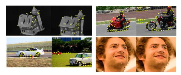
Figure 2.7: Examples of keypoints that represent an object inside an image. The keypoints become the vertices in the graph (Lê-Huu and Paragios, 2017; Zhou et al., 2013).
