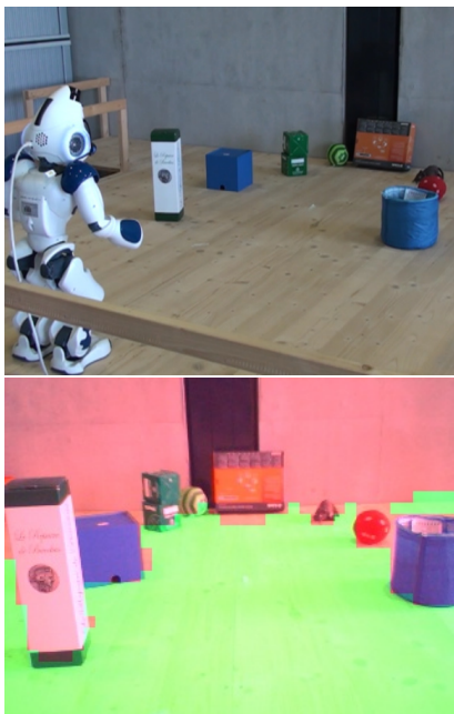
Figure 2.18: Example of learned traversability from [115], where collision-free zones are in green, otherwise red.
