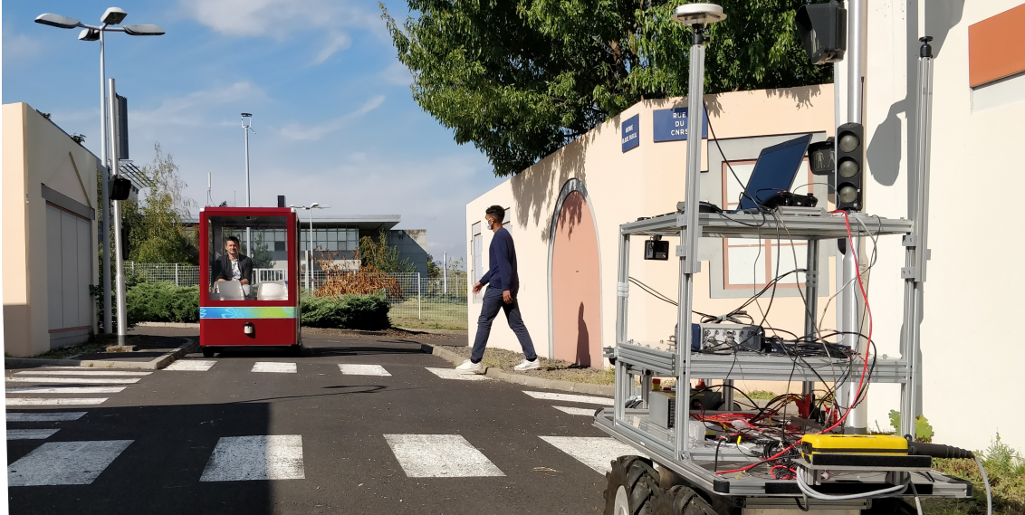
Figure 6.1: Example of an urban scenario that the robot can encounter. A pedestrian is crossing the road, while a vehicle is approaching the robot in the other lane. Using the Dynamic Lambda-Fields, the robot is able to estimate the risk of its actions, taking into account a generic risk that can be adapted depending on the scenario.
