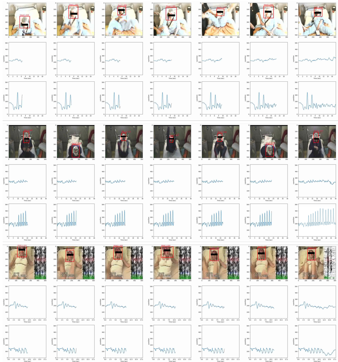
Figure 4.3: Selected samples of the head detection and the head movement trajectory from the cases in Fig. 4.1. For each demonstration, the first row is the image sequence of the seizure video with head detected. The second/third rows represent the horizontal/vertical coordinates of the center of the detected bounding box throughout the whole seizure event. Cyclic patterns are more obvious in the vertical directions, as the antero-posterior rocking movements are mainly perpendicular to the camera.
