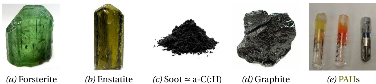
FIGURE I.10 – Appearance of various minerals. The (a) and (b) images show crystalline silicates. The soot powder (c) is an approximate analog of a\text{-C}(:\text{H}) , on the a\text{-C} end, except that soot can contain radicals with O, N, etc. These images are useful to visualize the differences in optical properties of these compounds. They however show macroscopic samples. Even the powder in image (c) is made of particles much larger than 1\ \mu\text{m} , which is the maximum size of interstellar grains. Credit: (a) forsterite from Rob LAVINSKY, licensed under CC BY-SA 3.0; (b) enstatite from Rob LAVINSKY, licensed under CC BY-SA 3.0; (c) soot from Wikipedia, not licensed; (d) graphite from Rob LAVINSKY, licensed under CC BY-SA 3.0; (e) PAHs from the Astrochemistry Lab, NASA Ames Research Center, with permission from Lou ALLAMANDOLA.
