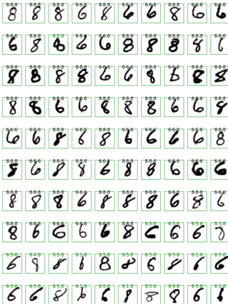
Figure 5.10: Training results of G(6,8) . Each image has three numbers from left to right: Label, Initial cluster assignment from IDEC, assignment after training with IDEC-LK. Black numbers mean that the initial assignment satisfies G(6,8) constraint. All of them do not change after the training. Green text is for the images that have changed their assignments to meet the requirement.
