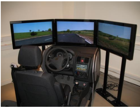
(a) Fixed-base driving simulator.
