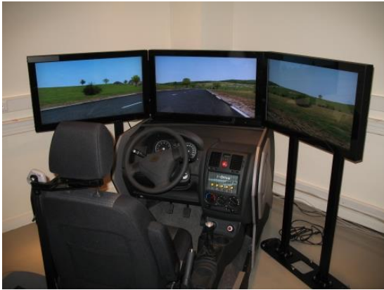
(a) Driving simulator SCANeR.
