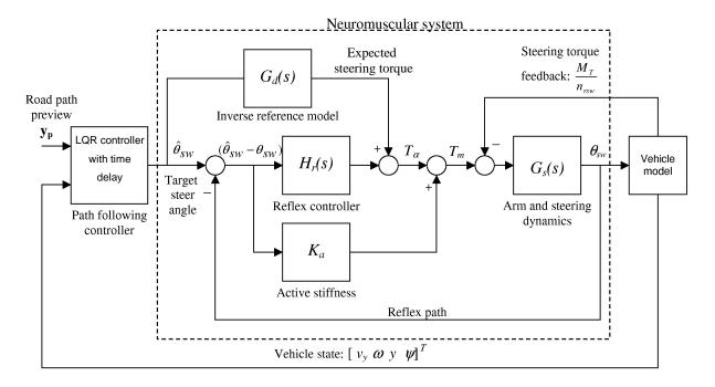
Figure 2.4 – Structure for driver path-following model with neuromuscular dynamics incorporated[10].
