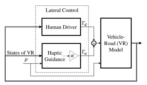
Figure 9.1 – Shared control between the human driver and haptic guidance system.  $\rho$ : road curvature;  $\alpha$ : sharing level;  $\Gamma_d$ : driver steering torque;  $\Gamma_a$ : haptic guidance torque.
