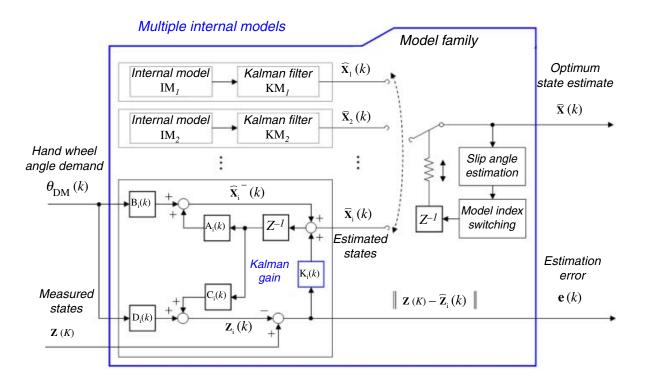
Figure 2.6 – State estimation using multiple models and Kalman filters[13].
