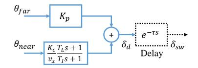
Figure 8.5 – Visual model with delay for identification.
