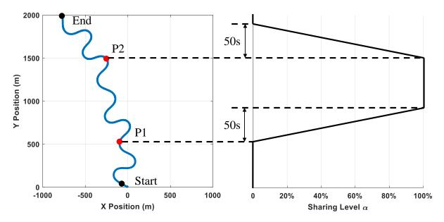
Figure 9.6 – Left: track used in the validation II; Right: variation of the sharing level in the experiment.
