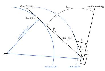
Figure 8.6 – Approximation of the far point angle and the near point angle.
