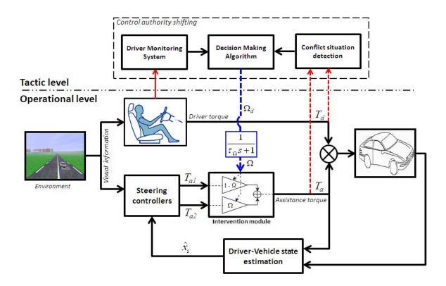
Figure 1.4 – Design of haptic guidance system proposed in  $[18] \odot 2013$  IEEE.
