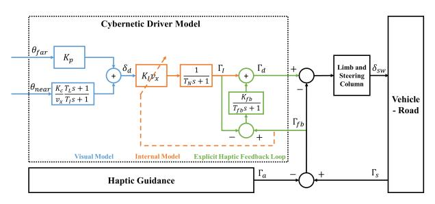
Figure 8.2 – Structure of the proposed cybernetic driver model. Blue: two-point visual model; Orange: driver internal model; Green: direct haptic feedback loop.
