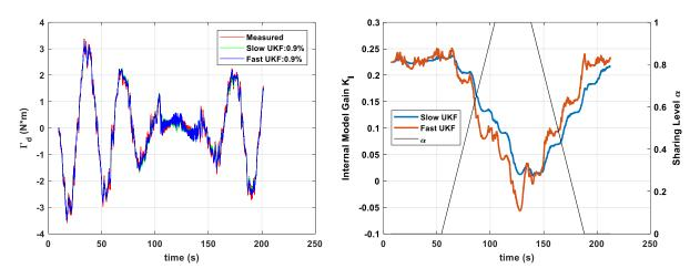
by the friction in the steering system that was measured by the torque sensor.
