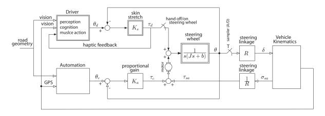
Figure 1.3 – Design of haptic guidance system proposed in [17]  $\bigcirc$  2004 IEEE. Equation numbers in the "Automation" and "Vehicle Kinematics" boxes are removed.
