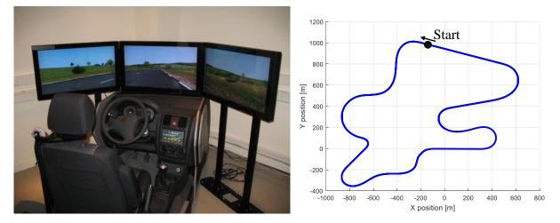
Figure 9.3 – Left: fixed-base driving simulator; Right: track used in the first experiment.
