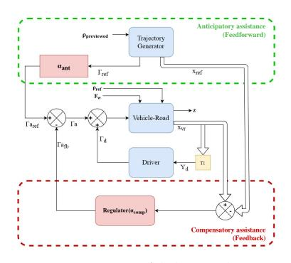
Figure 8.4 – Design strategy of the haptic guidance system.
