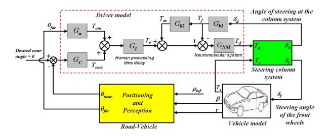
Figure 2.5 – The structure of the driver model [12]  $\odot$  2009 IEEE.
