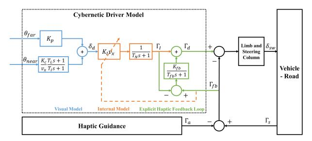
Figure 9.2 – Structure of the proposed cybernetic driver model. Blue: two-point visual model; Orange: driver internal model; Green: direct haptic feedback loop.
