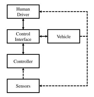
Figure 1.2 – Shared control architecture proposed in [12]. Solid line: power exchange; Dashed line: signal or information exchange.
