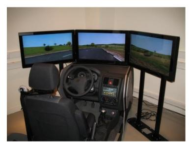
Figure 3.1 – Fixed-based driving simulator.
