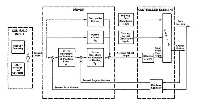
Figure 2.1 – Topology of the driver/vehicle system combining open- and closed-loop precognitive, pursuit, and compensatory control structures [3]  $\bigcirc$  1977 Sage Publications.
