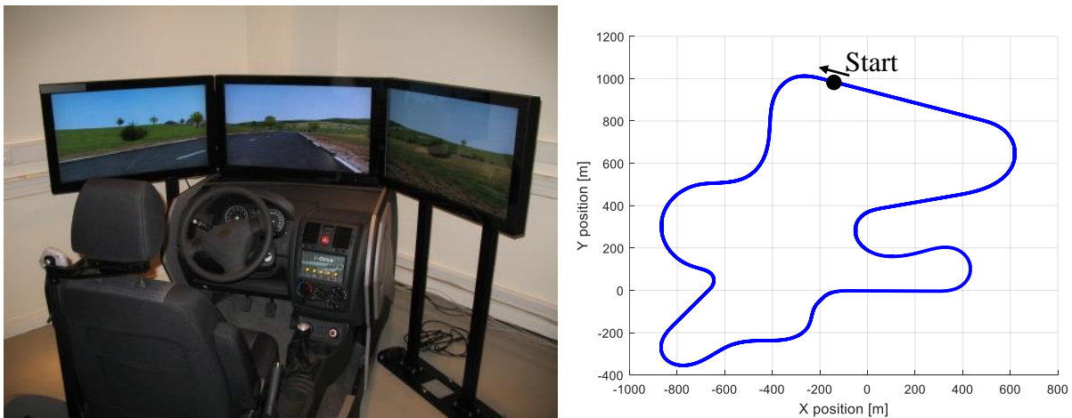
Figure 9.3 – Left: fixed-base driving simulator; Right: track used in the first experiment.
