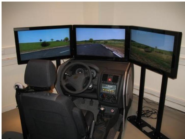
Figure 3.1 – Fixed-based driving simulator.
