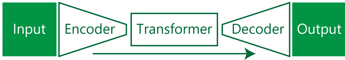
Figure 4.6 – A transformer working on latent codes produced by an encoder. The transformer outputs updated latent codes that are then decoded back into the input space. The addition of an encoder and decoder should unburden the transformer during training.
