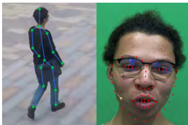
Figure 1.10 – Left) Landmarks for body joints on the previous example in Figure 1.8. Right) An example of facial landmarks detection using DLib.
