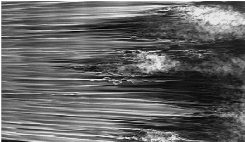
Figure 2.2: Smoke visualization of streamwise streaks appearing in a boundary layer subjected to moderate level of freestream turbulence intensity Tu = 2.2\% . The flow, coming from the left, is captured at a certain distance from the leading edge and it transitions (breakdown and turbulence spot formations) in the right edge of the image. Figure reproduced from Matsubara et al. , [26].
