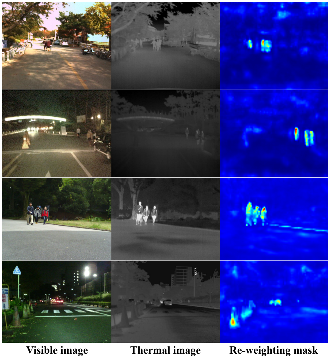
FIGURE 5.11 – Visualization of the visible-thermal image pairs and the 2-D spatial re-weighting masks from the proposed F-MSE loss. The first two lines of multispectral images pairs come from KAIST dataset, and the last two lines come from MFNet dataset.
