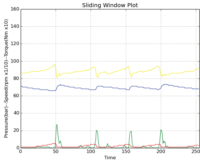
Figure 19. Pressure loop at 70 bar with an inefficient pump.
