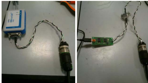
Figure 8. (left) IXXAT USB to CAN, (right) open-source Serial to CAN.
