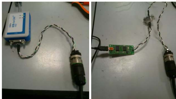
Figure 8. (left) IXXAT USB to CAN, (right) open-source Serial to CAN.
