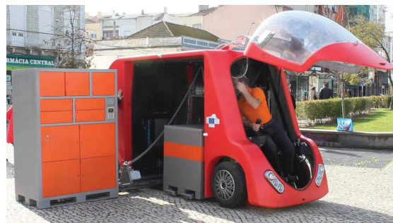
Figure 1. FURBOT while loading freight.
